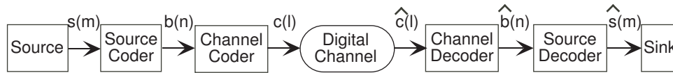
Figure 6.20: To correct errors that occur in the digital channel, a channel coder and decoder are added to the communication system. Properly designed channel coding can greatly reduce the probability (from the uncoded value of p_e ) that a data bit b(n) is received incorrectly even when the probability of c(l) be received in error remains p_e or becomes larger. This system forms the Fundamental Model of Digital Communication.
