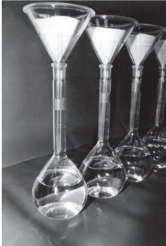
Figure 4.2 Separation of silica from the concrete extracts.
