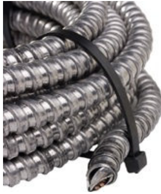
Figure 4.57 Electric motors often vibrate whilst operating, which is why their final connections are often wired with flexible conduit
