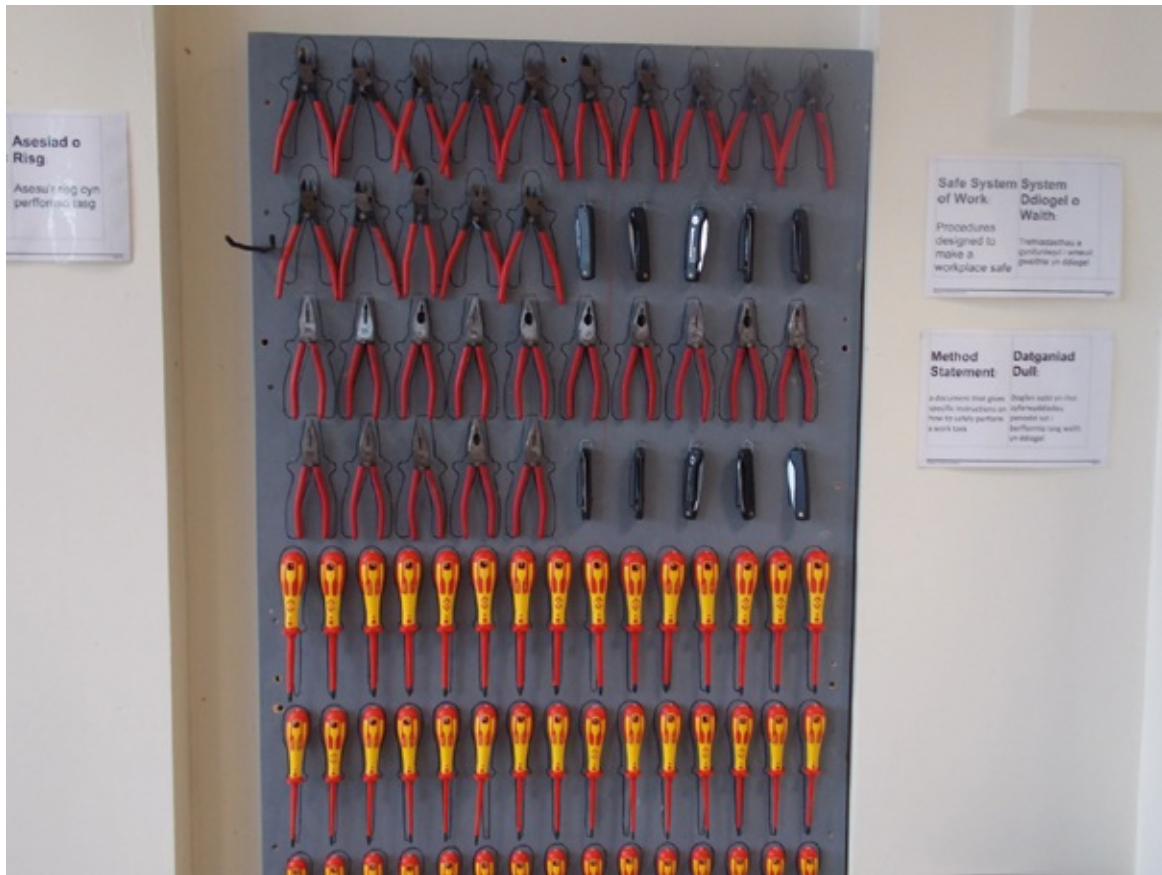
Figure 1.6 Shadow boards indicate when a tool is missing or lost
