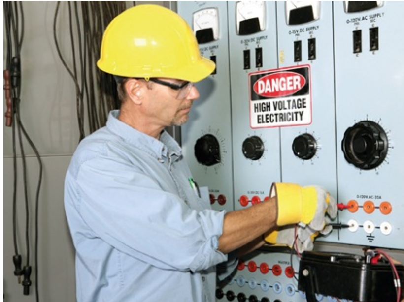
Figure 1.16 Some electricians' gloves can withstand voltages as large as 36,000 volts
