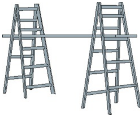
Figure 1.29 A trestle scaffold is very useful if the work surface happens to be uneven
