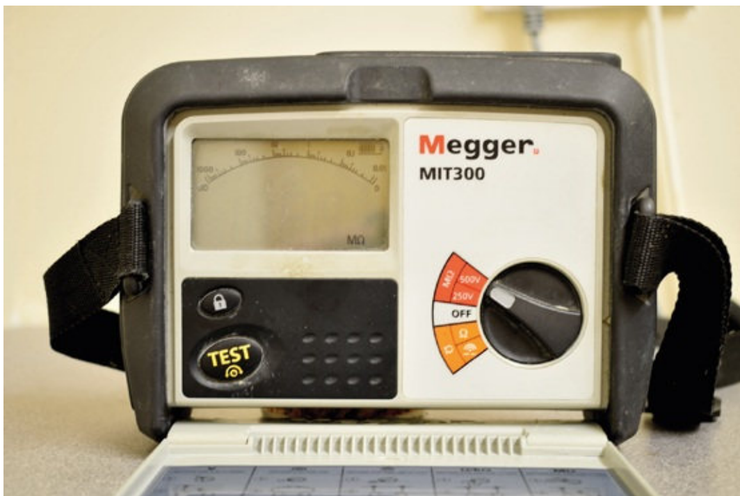
Figure 4.60 The M \Omega sign indicates Insulation Resistance
