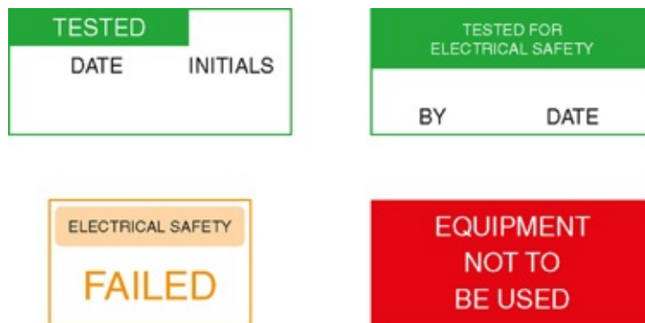
Figure 1.25 Labels can prove that a piece of electrical equipment have been electrically tested or highlight that it is Not to be used
