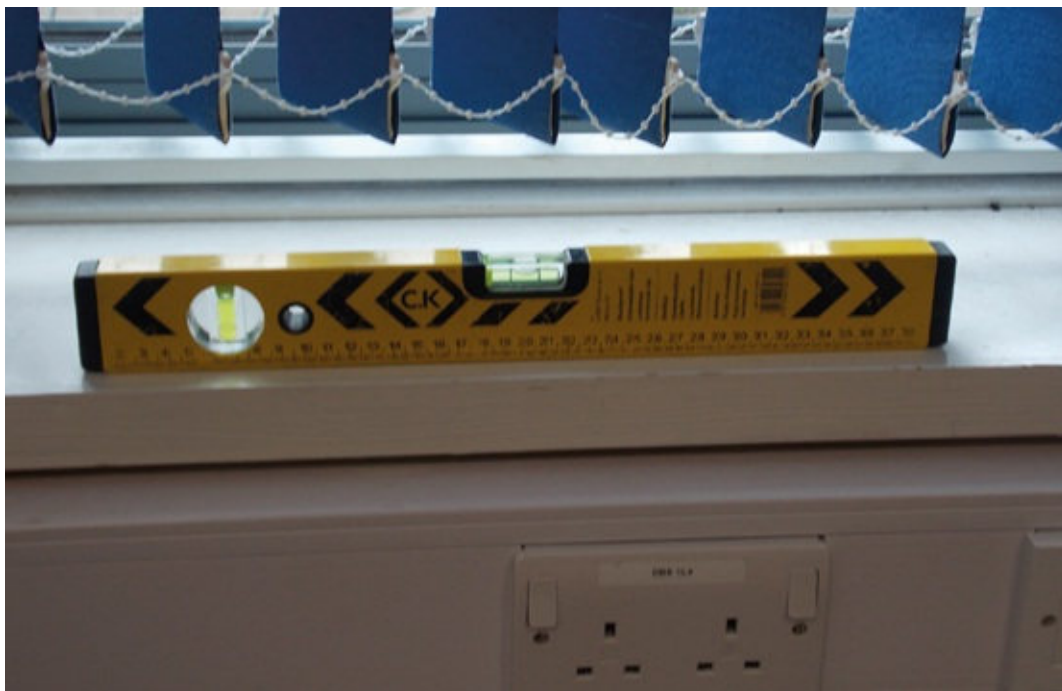
Figure 4.1 Spirit levels are very useful to ensure that work surfaces or aspects of electrical installation are parallel and even
