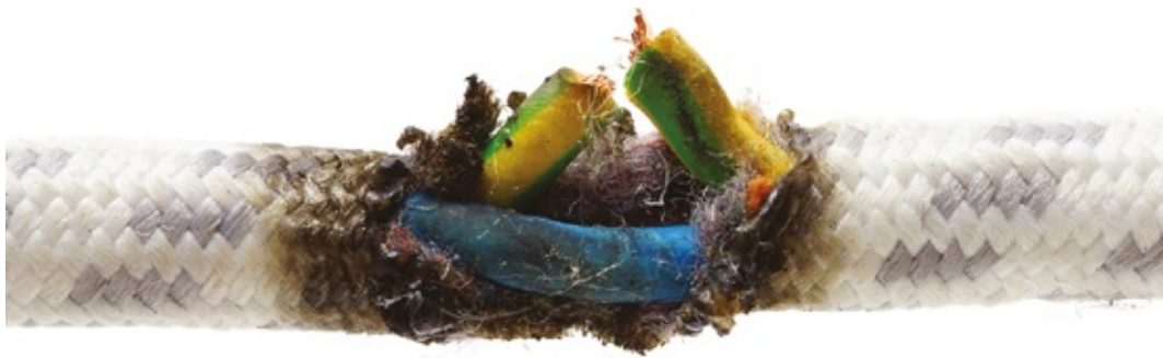
Figure 1.24 Overheating can lead to electrical fires
