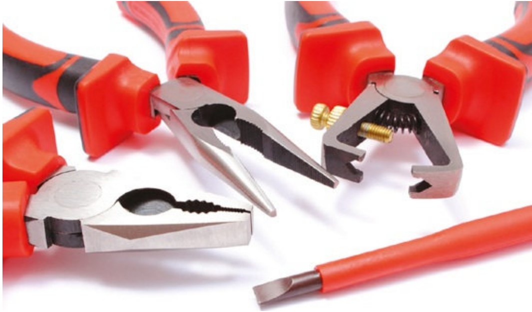
Figure 4.2 An electrician's tools should be insulated along the majority of their length
