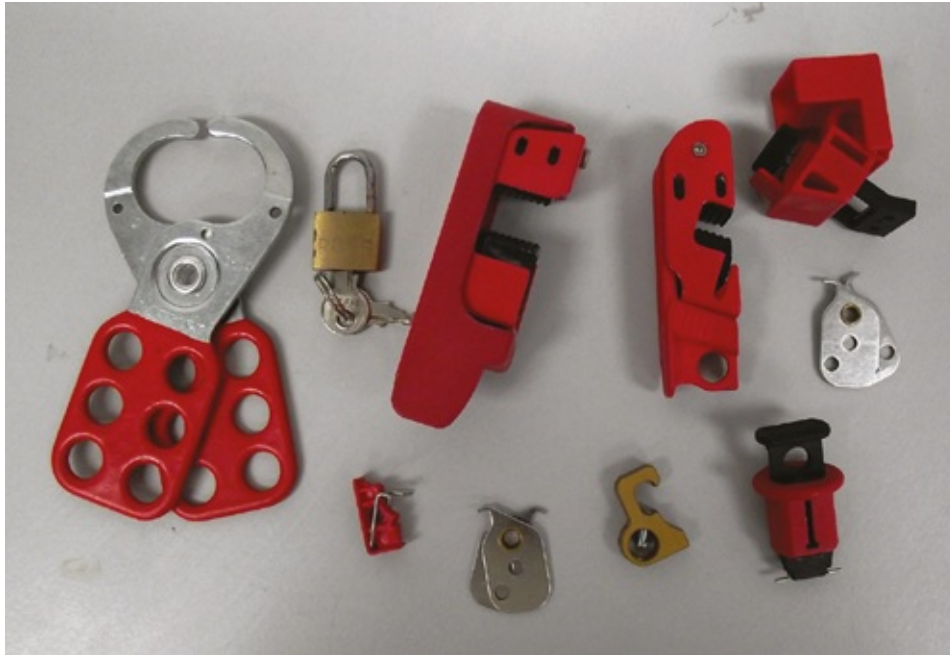
Figure 1.27 Electrical circuits need to be locked off to ensure that the electrical supply is not accidentally switched back on
