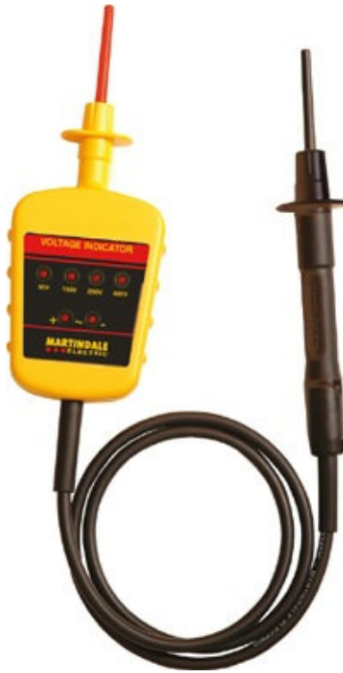
Figure 1.26 Only Approved Test equipment is permitted to ensure that an electrical circuit has been made dead
