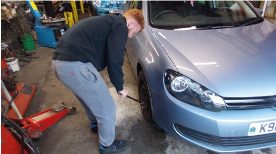
Figure 4.4 The final part of changing a tyre involves using a torque wrench which has been set to an optimum amount of force to tighten the wheel nuts
