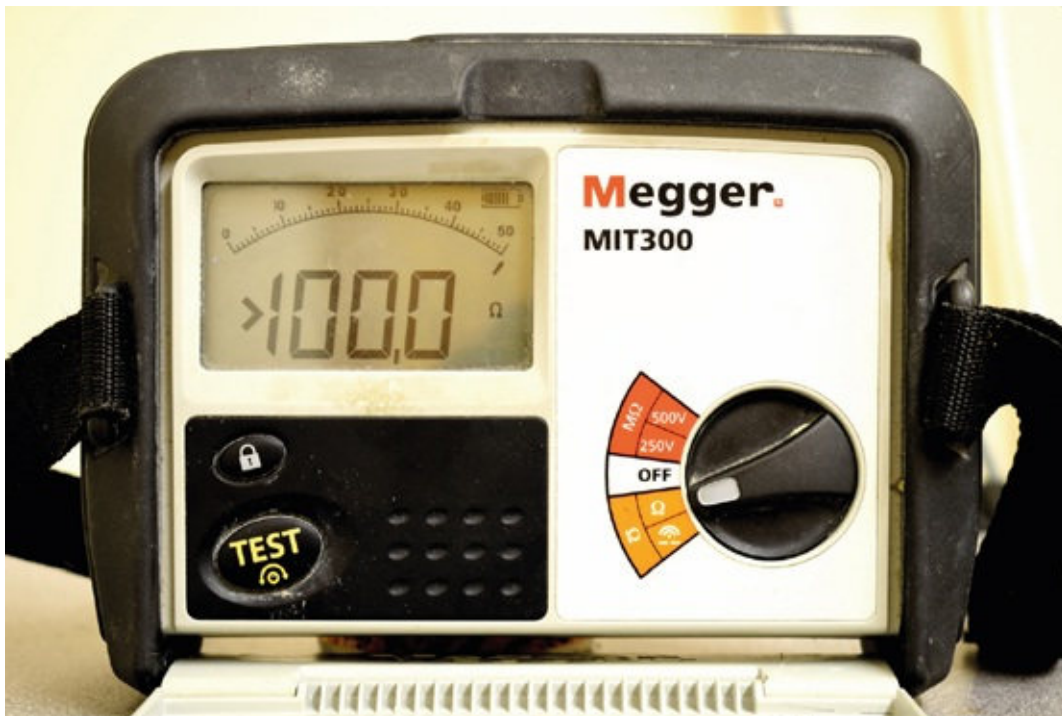
Figure 4.59 The \Omega sign indicates Resistance
