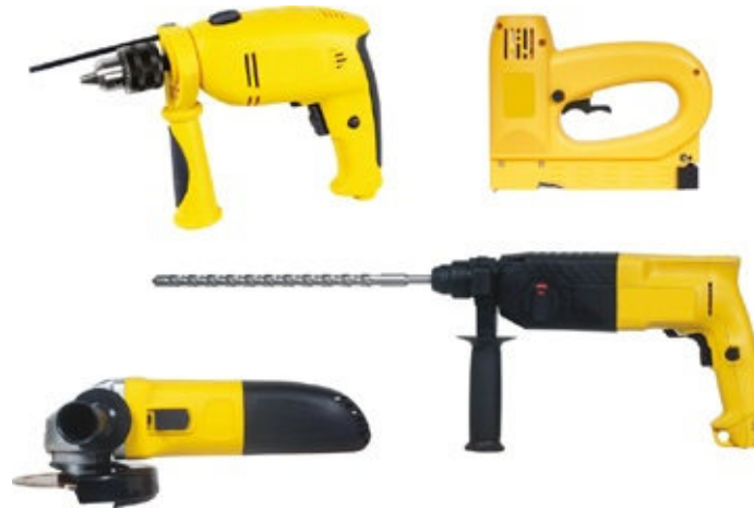
Figure 4.7 A wide variety of power tools are used on site, but they all must be registered, inspected and tested before use
