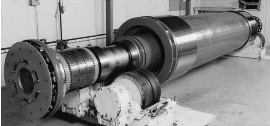
Figure 4.9 Rotor of a 100-MW turbine generator. A brushless excitation system, used to supply dc field current, is seen on the near end of the rotor. ( Photo courtesy of General Electric Company. )
