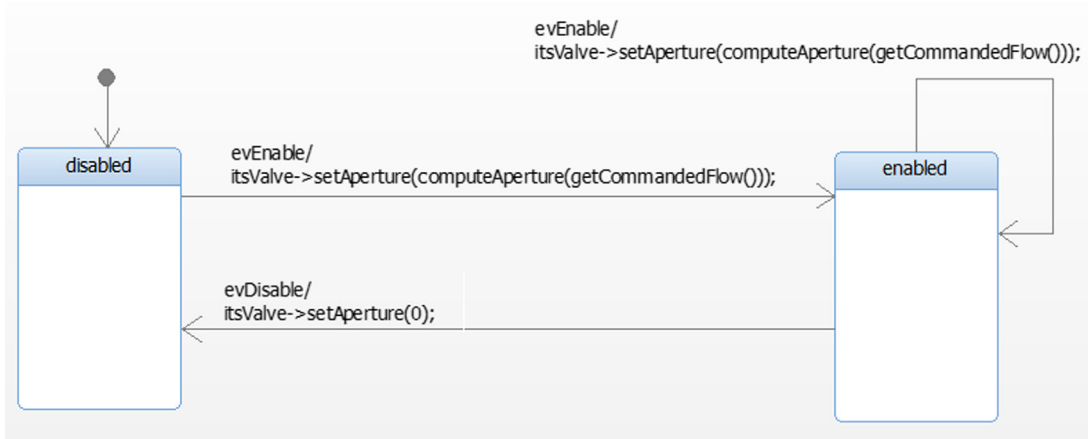
Figure 7.8 State machine for the Gas class.
