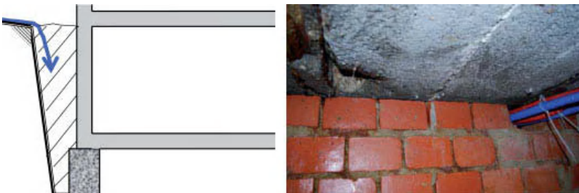
Figure 5.20. Seeping rainwater wedge around a basement.
