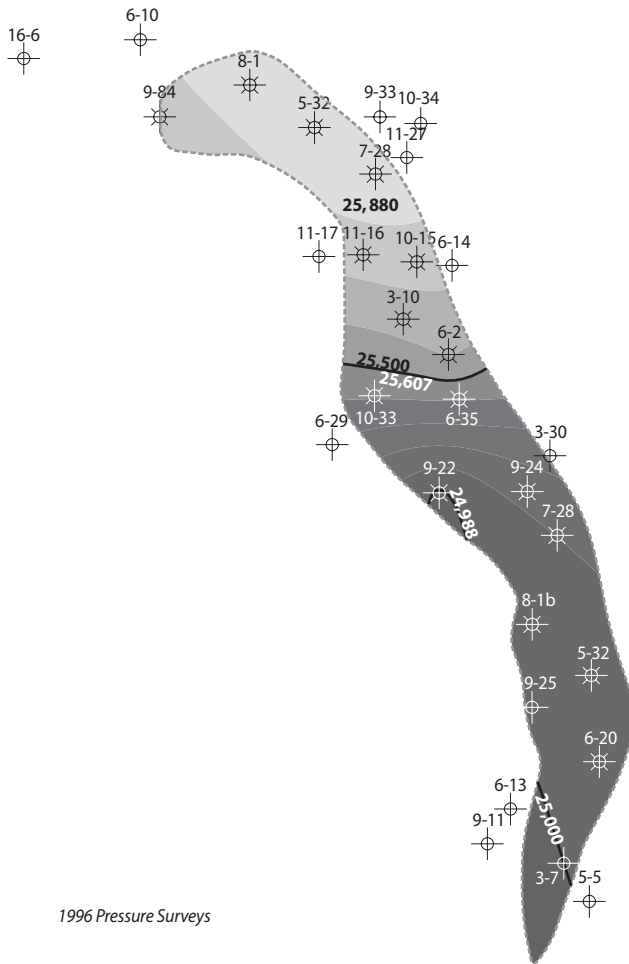
Fig. 5-17 Reservoir Pressure Contours—Gas Reservoir, 1996
