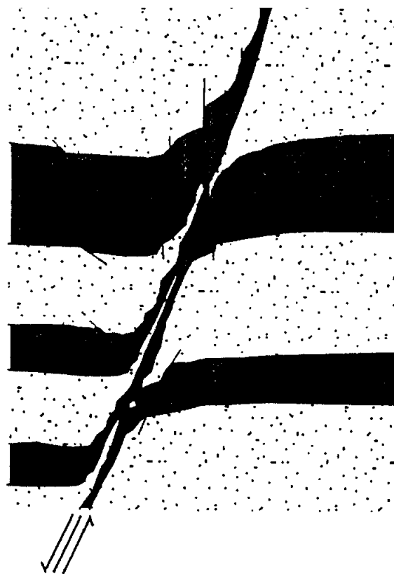
Fig. 3–32 Fault Gouge (Smear) May Provide Seal
