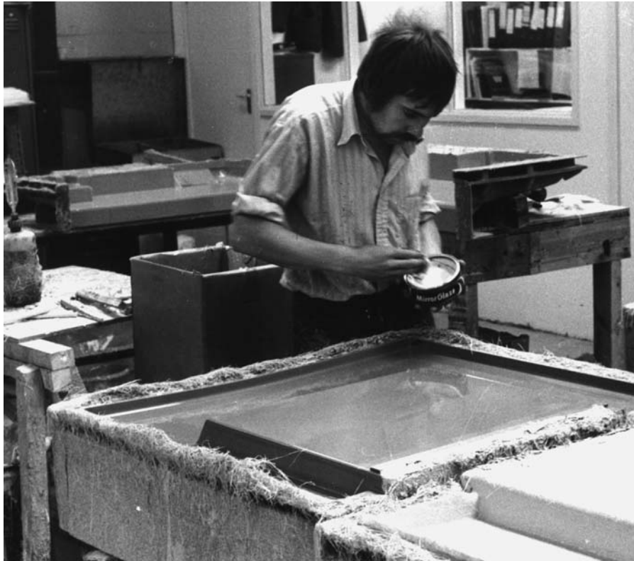
3.3 Mould waxing prior to moulding.
