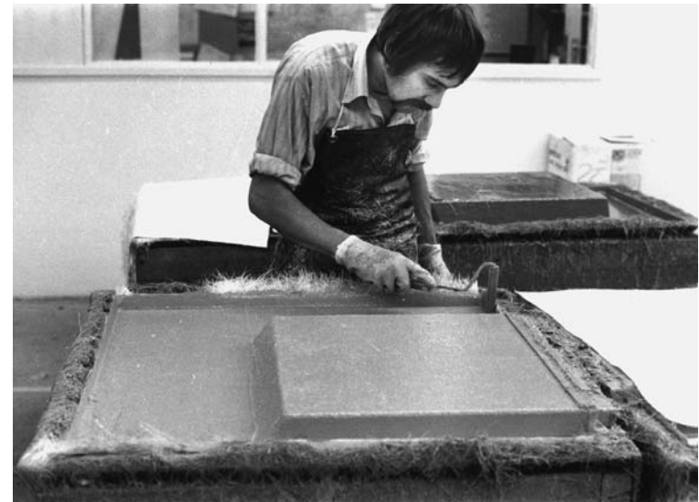
3.4 Rolling out the lay-up to remove air bubbles.
