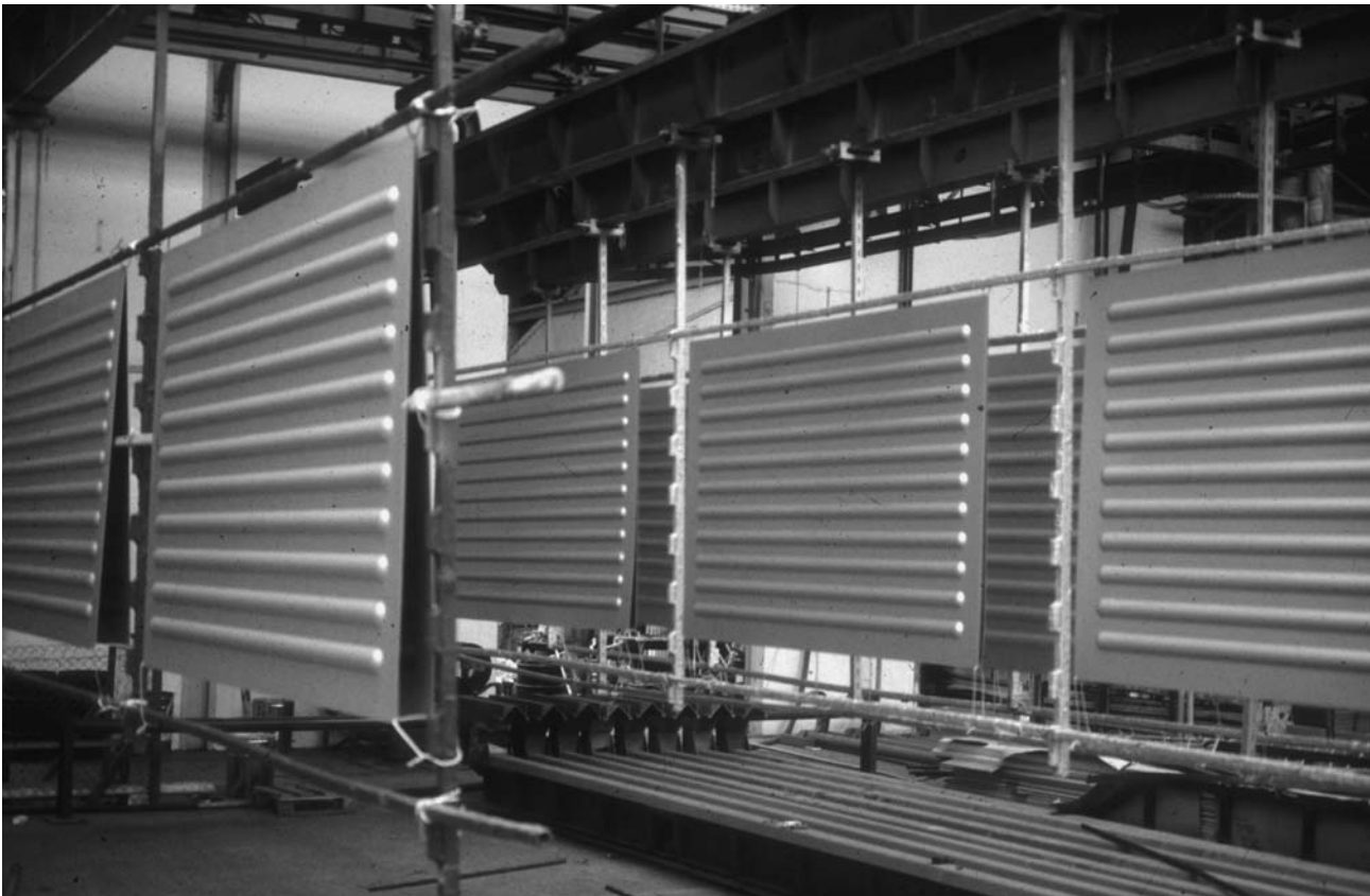
6.33 Panels for Gatwick Airport on Duranar coating line.
