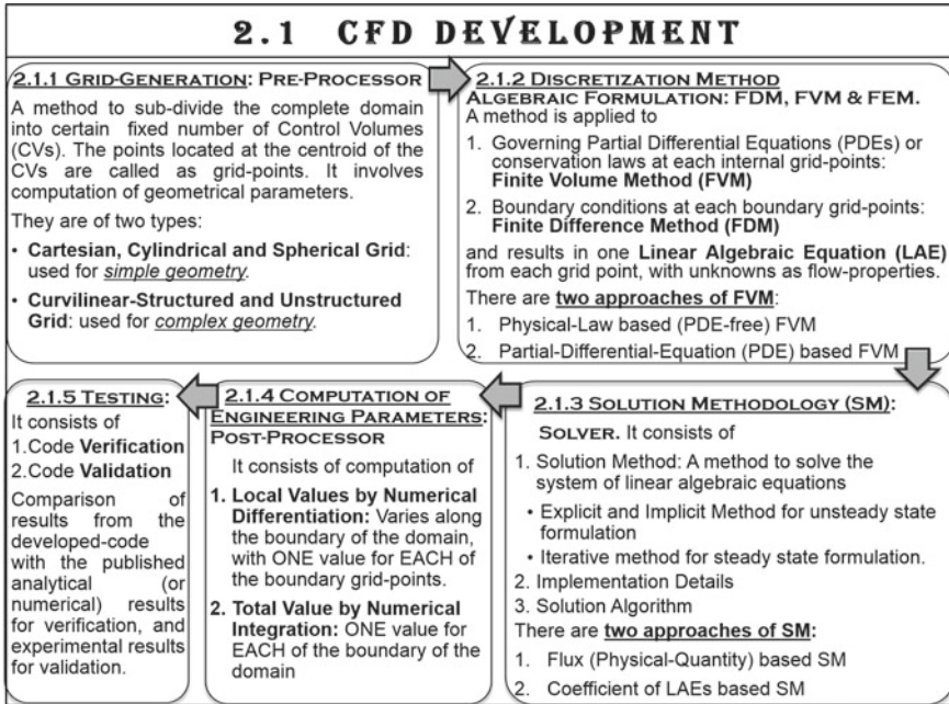
Fig. 2.1 Schematic description of five different steps of CFD development
