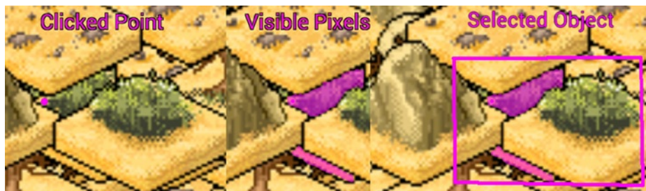
Figure 5-4. The results of a pixel-perfect picking. Users can select sprites which may be complex or hidden under other objects in Z-ordering
