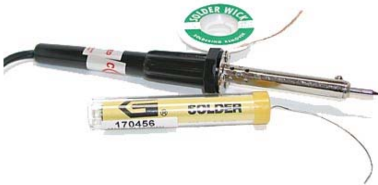
Figure 40: Cheap soldering iron, solder and wick from JAMECO
