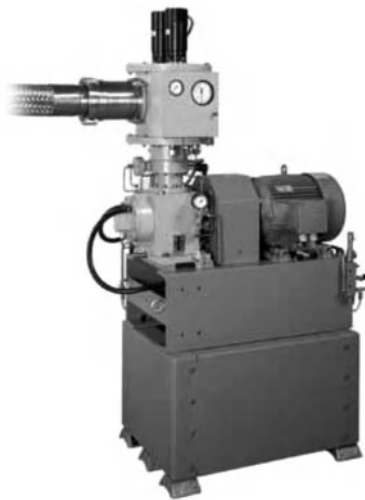
Figure 9.22 Two-stages and single-cylinder of Stirling refrigerators (Reproduced with permission from Stirling Cryogenic BV, //www.stirlingcryogenics.com/products/cryogenic-cooling (accessed October 29, 2012)).
