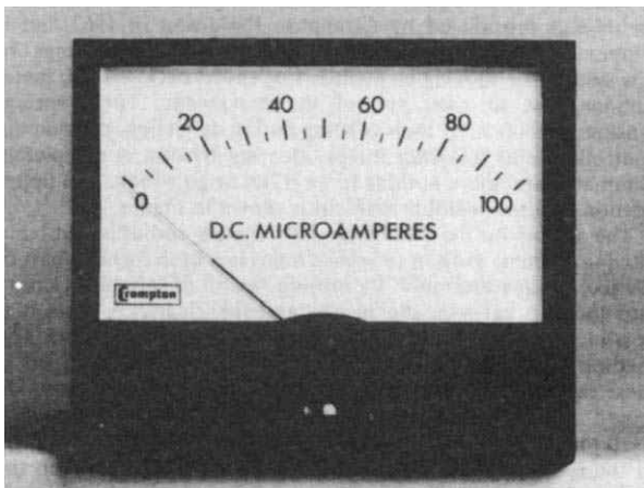
Figure 18.3 A microamp panel meter incorporating taut-band suspension (Crompton Instruments)
