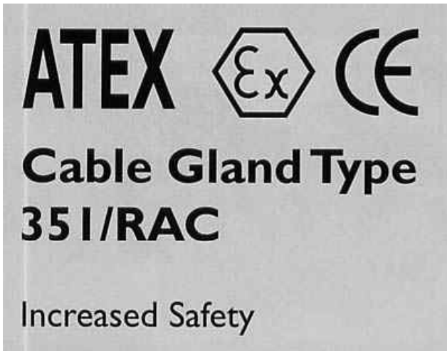
Figure 23.3 Typical ATEX compliance marking (CEAG Crouse Hinds)
