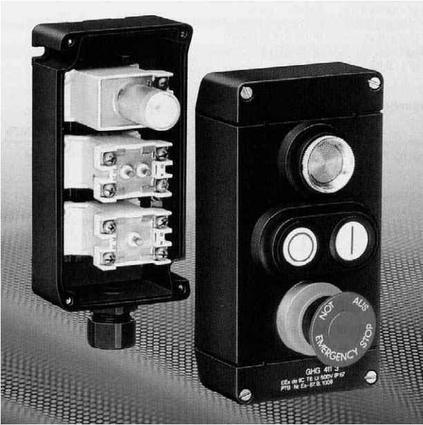
Figure 23.7 Explosion protected EEx 'e/d' control station (Enclosure EEx 'e'. Switches and indicator lamp EEx 'de') (CEAG Crouse Hinds)
