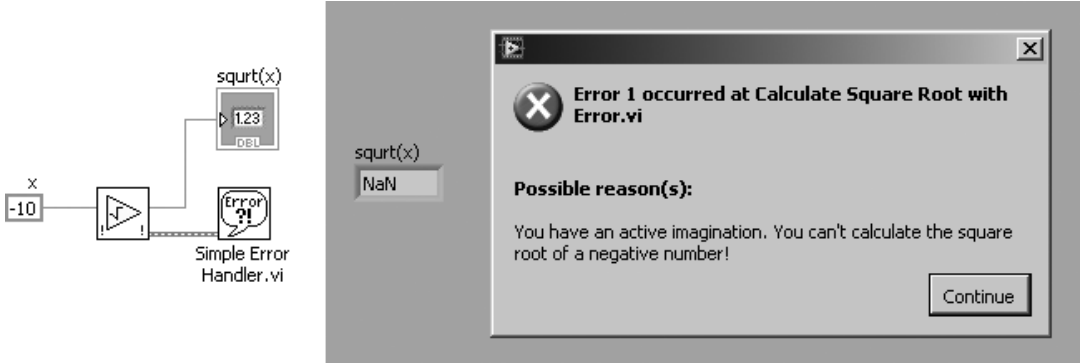
Figure 7.75 Calling Calculate Square Root with Error.vi as a subVI
