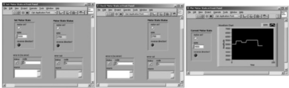
Figure 13.63 Three subVIs that use the Motor State cluster
