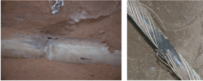
Figure 13.25 Cable and conduit damage observed from rocket-triggered lightning flashes above the ground. (From Electric Power Research Institute. Copyright © 1993. Reprinted with permission.)
