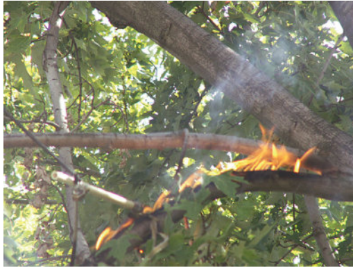
Figure 14.28 Open flame on a silver maple branch energized at 7.6 kV. (From EPRI 1016219, Optimal Design of Overhead Distribution Systems: Understanding Touch Voltage Potential Risks Due to Tree-to-Conductor Contacts on Distribution Circuits , Electric Power Research Institute, Palo Alto, CA, 2007. Copyright 2007. Reprinted with permission.)
