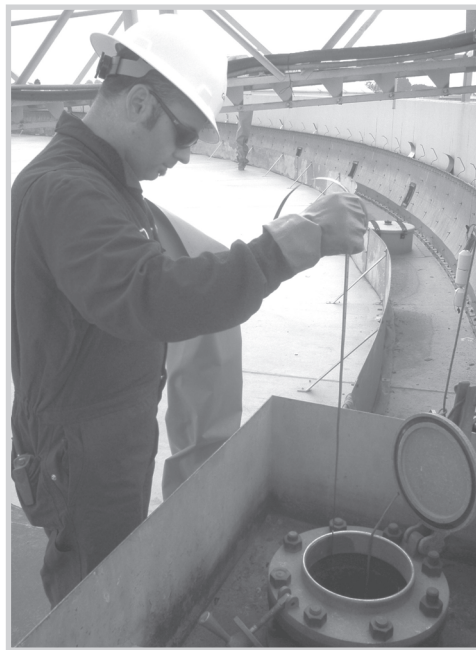
Fig. 4-1. Gauging a crude oil tank. The gauger reads the tape, much like reading the dipstick in a car.
