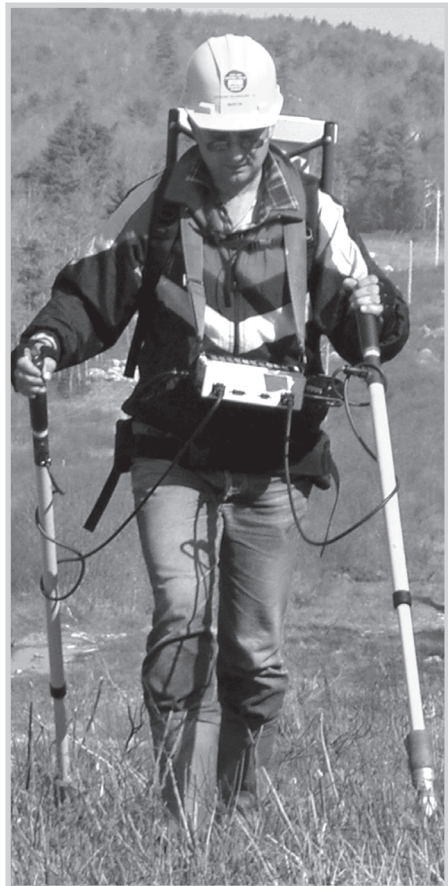
Fig. 9–20. CIPS surveyor walking the pipeline (Courtesy Cathodic Technology Limited)
