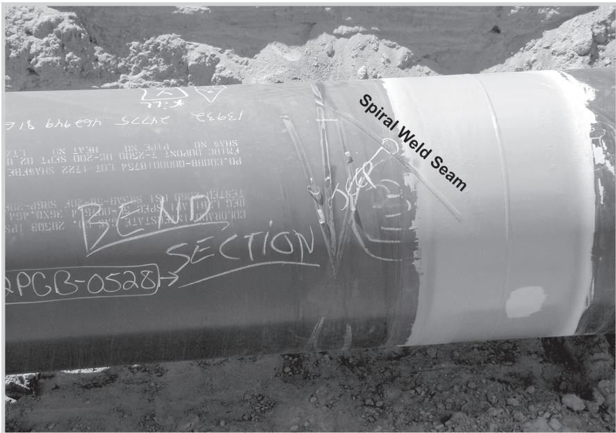
Fig. 11-1. Spiral welded pipe. The weld seam is visible next to the girth weld. (Courtesy U.S. Pipeline, Inc.; photo by Adam Aronson)
