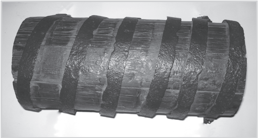
Fig. 2-2. Segment of hollowed log used as a gas pipeline joint (Courtesy Midwest Energy Association; photo by Tom Miesner)
