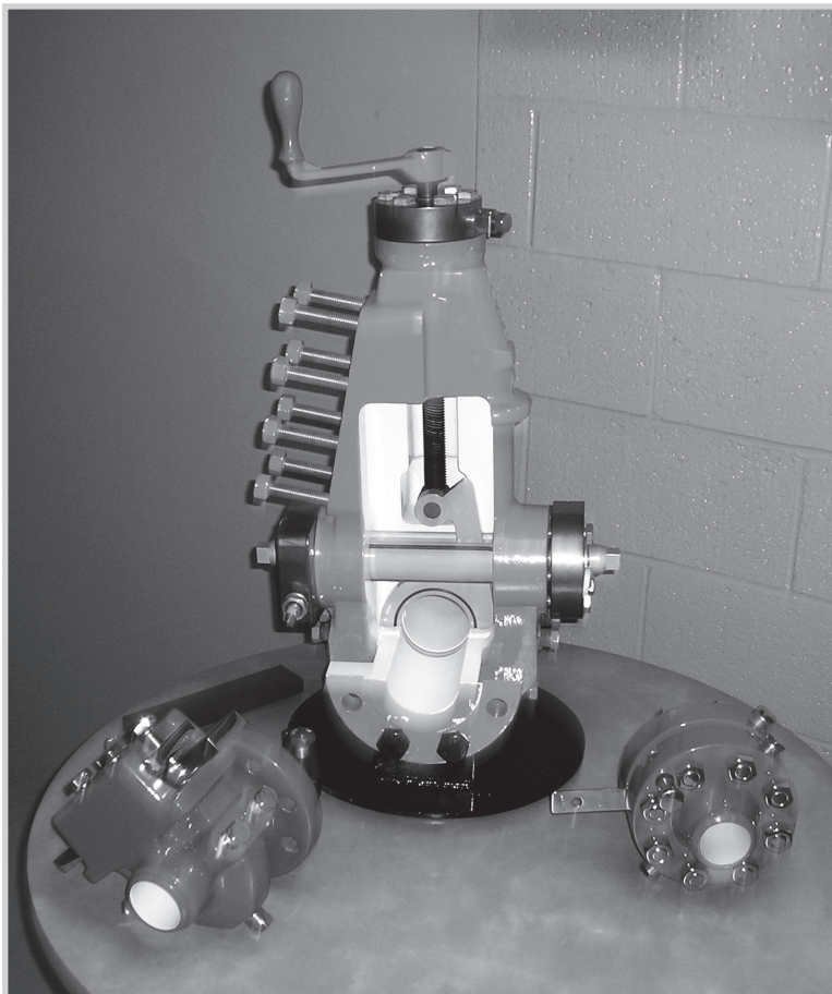
Fig. 11–26. Orifice plate holders. The orifice plate carrier in the middle allows the orifice plates to be changed without shutting down the line. The crank lifts the plate carrier above a shut-off valve. The valve is shut, and the orifice plate is changed. Then the valve is opened, and the orifice plate is reinserted. The other two holders require shutting down the line to change the orifice plate. (Courtesy FMC Technologies)
