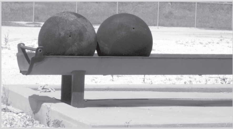
Fig. 9–30. Spheres waiting to be launched in a natural gas pipeline (Courtesy Miesner, LLC)
