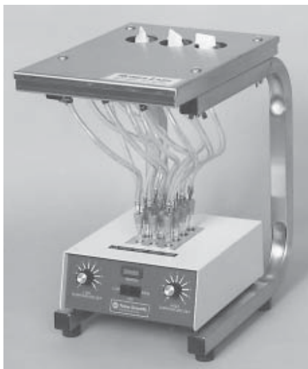
Fig. 4. Solvent Evaporation System.
