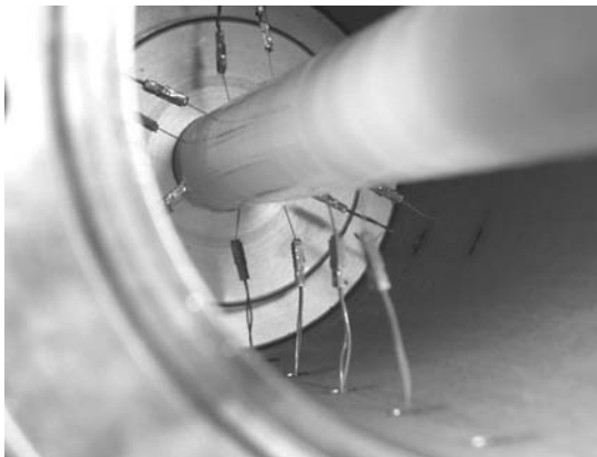
Fig. 24 MIRRAS sensors positioned for casting inside 6-in. hybrid motor assembly.
