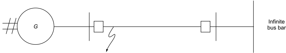
Fig. 8.100 A simple power system
