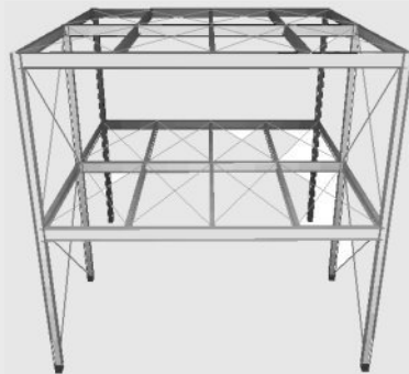
Figure 2.43 – Structural steel model with horizontal bracing
