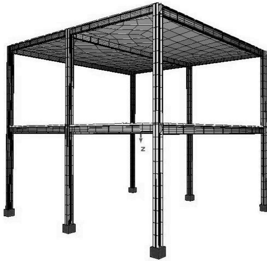
Figure 2.20 – Beam and shell structural model
