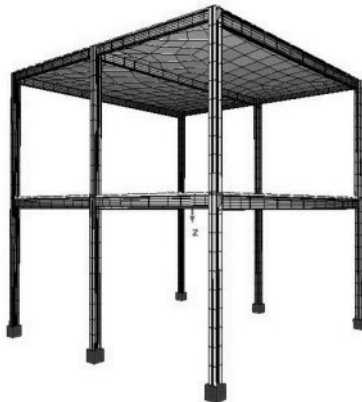
Figure 2.4 – Structural model with two-dimensional elements
