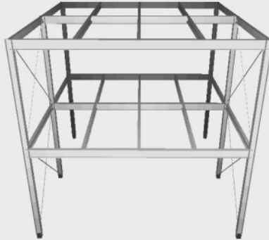
Figure 2.42 – Structural steel model (neglecting the slab)
