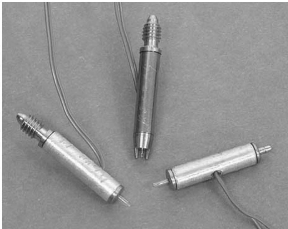
Fig. 1. Various configurations of piezoelectric microdispensing devices manufactured by MicroFab Technologies, Inc.
