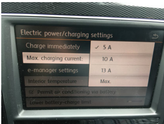
Figure 9.77 The option to set maximum charge current determines the charge time. The lower figure can be set, for example, when charging from solar panel output
