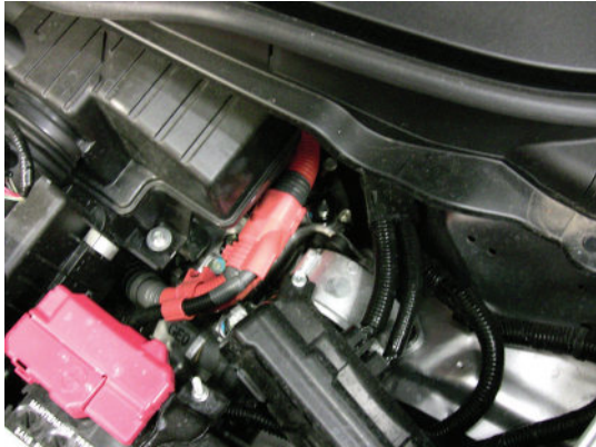
Figure 2.6 High-voltage cables are always orange
