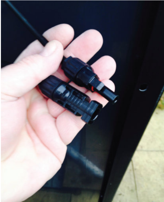
Figure 7.24 DC panel connections
