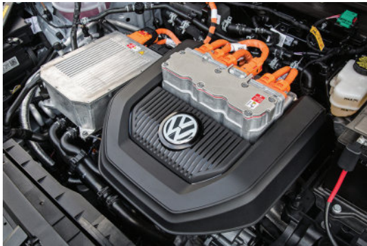
Figure 4.31 VW Golf-e showing some of the orange cables
