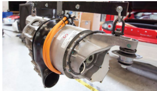
Figure 9.12 Tesla's AC induction motor (Source: Tesla Motors)
