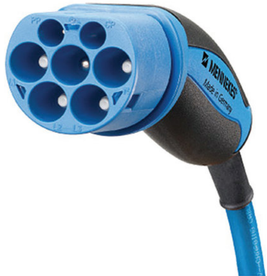
Figure 7.14 Type 2 plug. The pins from the top left and clockwise are: Proximity (PP), Control pilot (CP), Neutral (N), L3, L2, L1 and the Earth pin in the centre (Source: Mennekes)
