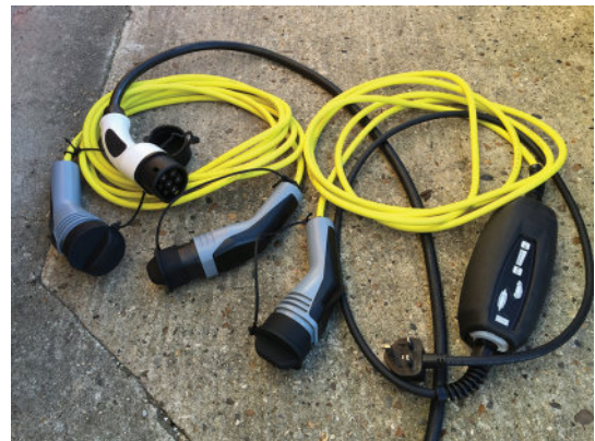
Figure 8.4 Domestic mains and charge point cables
