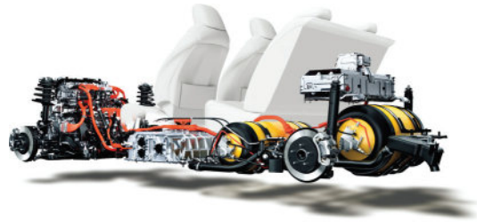
Figure 9.38 Cutaway view of the Mirai showing the fuel tanks in yellow (Source: Toyota Media)
