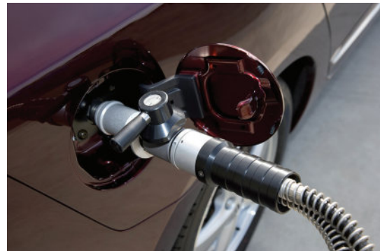
Figure 9.36 Fuelling pipe connection (Source: Honda Media)
