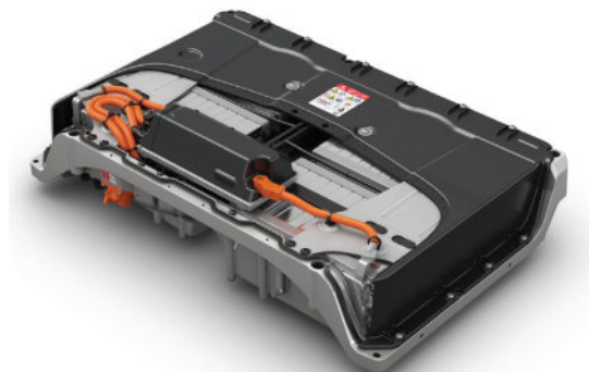
Figure 9.75 Battery pack: 120 kg and 96 lithium-ion cells results in 8.8 kWh at 345 V (Source: Volkswagen Media)
