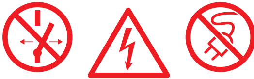
Figure 8.3 Warning signs used when work is being carried out on a vehicle after de-energization
