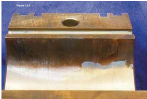
Figure 13.4 Varnish Formation on Plain Bearing and Shaft.
