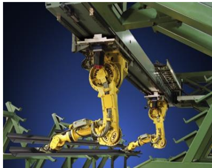
Figure 13-16. A robot on rails from the FANUC America Corporation, reproduced here for educational purposes.
