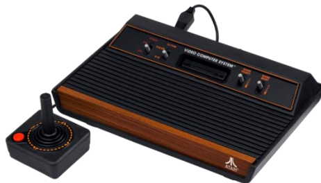
Figure 3-2. An Atari 2600 with separate instruction memory (ROM stored on cartridges) and data memory (RAM). (Wikipedia users Evan-Amos and Locke Cole)
