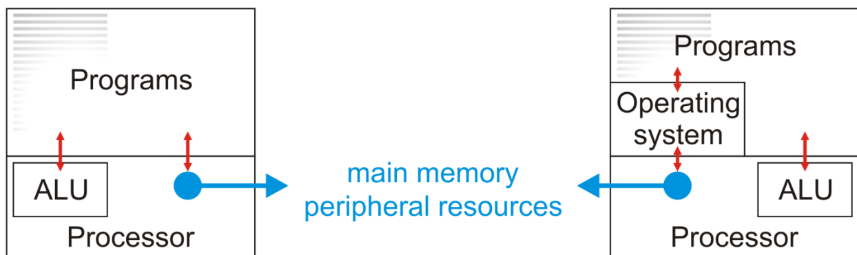
Figure 1-2. Configuration of smaller embedded systems versus larger embedded and general-purpose systems.
