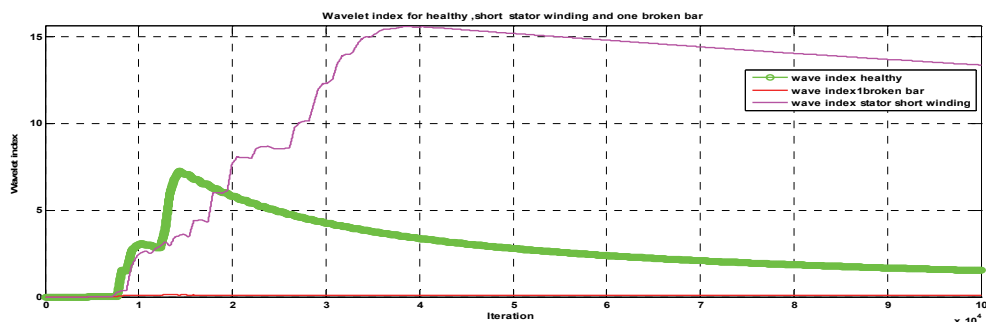
Fig. 14. Wavelet index for fault detection
