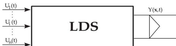
Fig. 2. Lumped-input and distributed-parameter-output system - LDS
