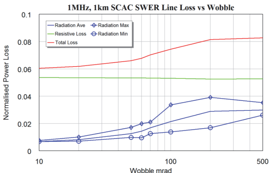
Fig. 3. Radiation loss of a SWER line with bends.
