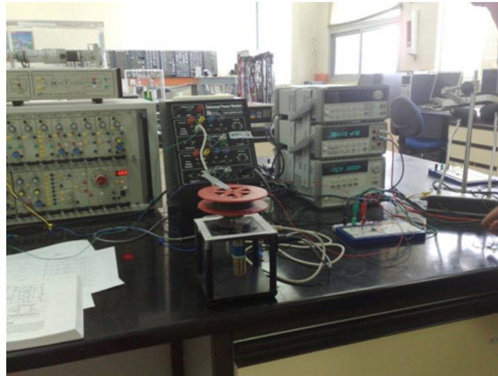
Figure 18. The setup of the light tracking servo system
