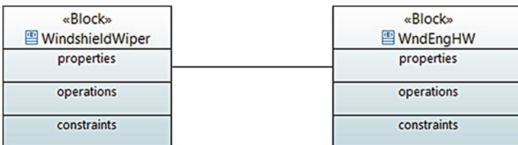
Fig. 2.6 An example principle—bidirectional coupling between two blocks
