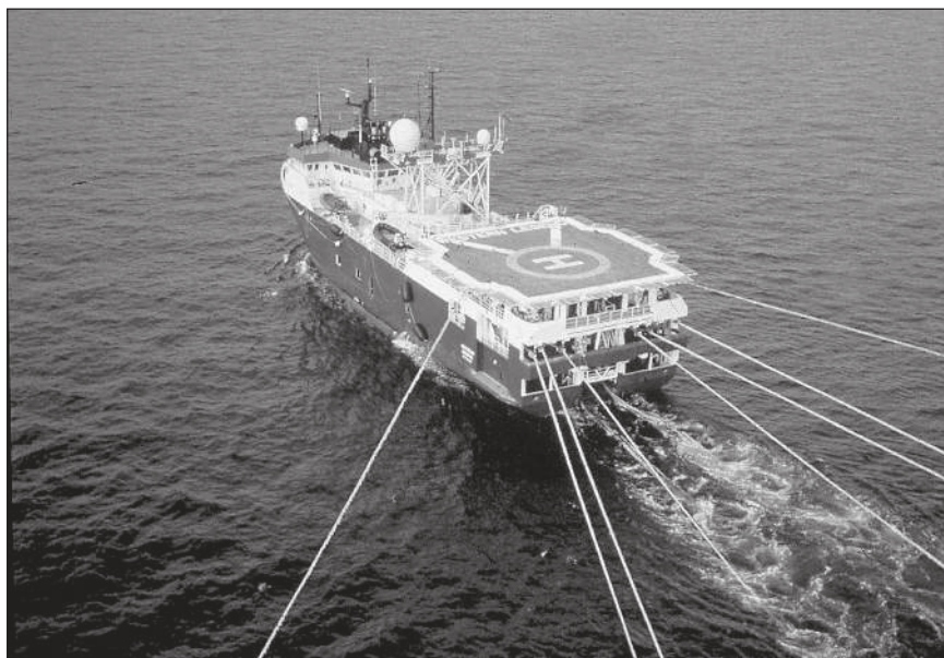
Plate 13–5. Seismic ship towing air gun arrays and streamers. (Courtesy of Western Geophysical Division of Baker Hughes.)
