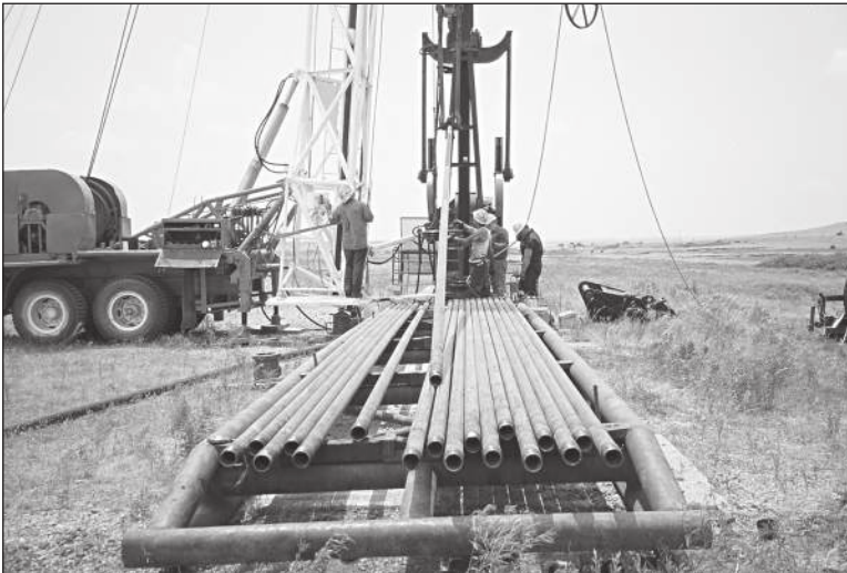
Plate 19–5. Tubing being run into a well
