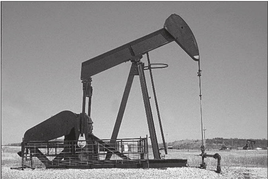
Plate 19–7. Artificial lift with a sucker-rod pumping unit
