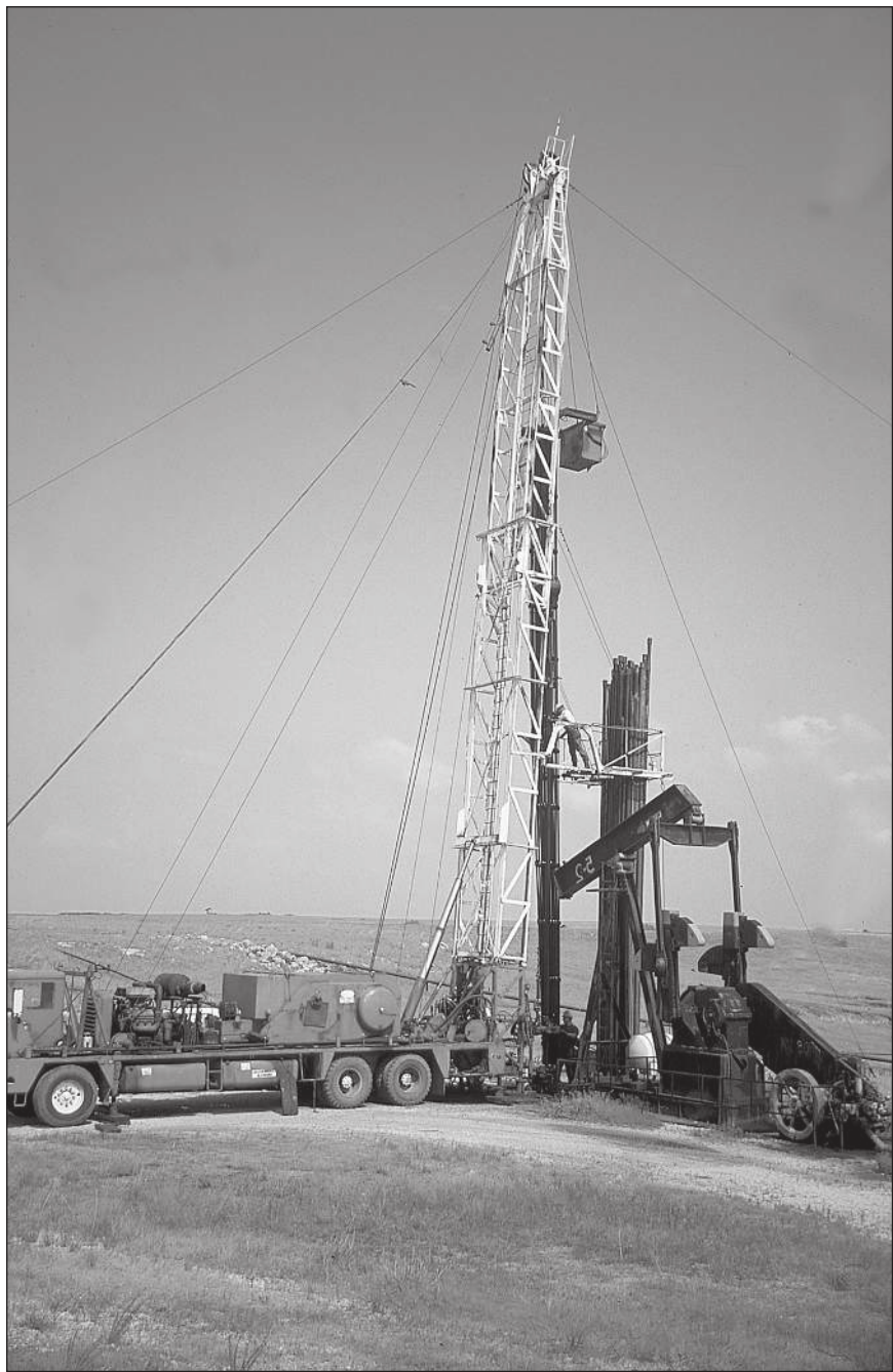
Plate 22–2. Well service unit with a structural mast that is pulling tubing. Note the tubing platform (lower) and rod basket (higher).
