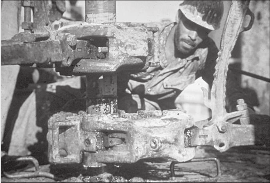
Plate 15–3. Tongs and spinning wrench being used on drillpipe. (Courtesy of API and Chevron.)
