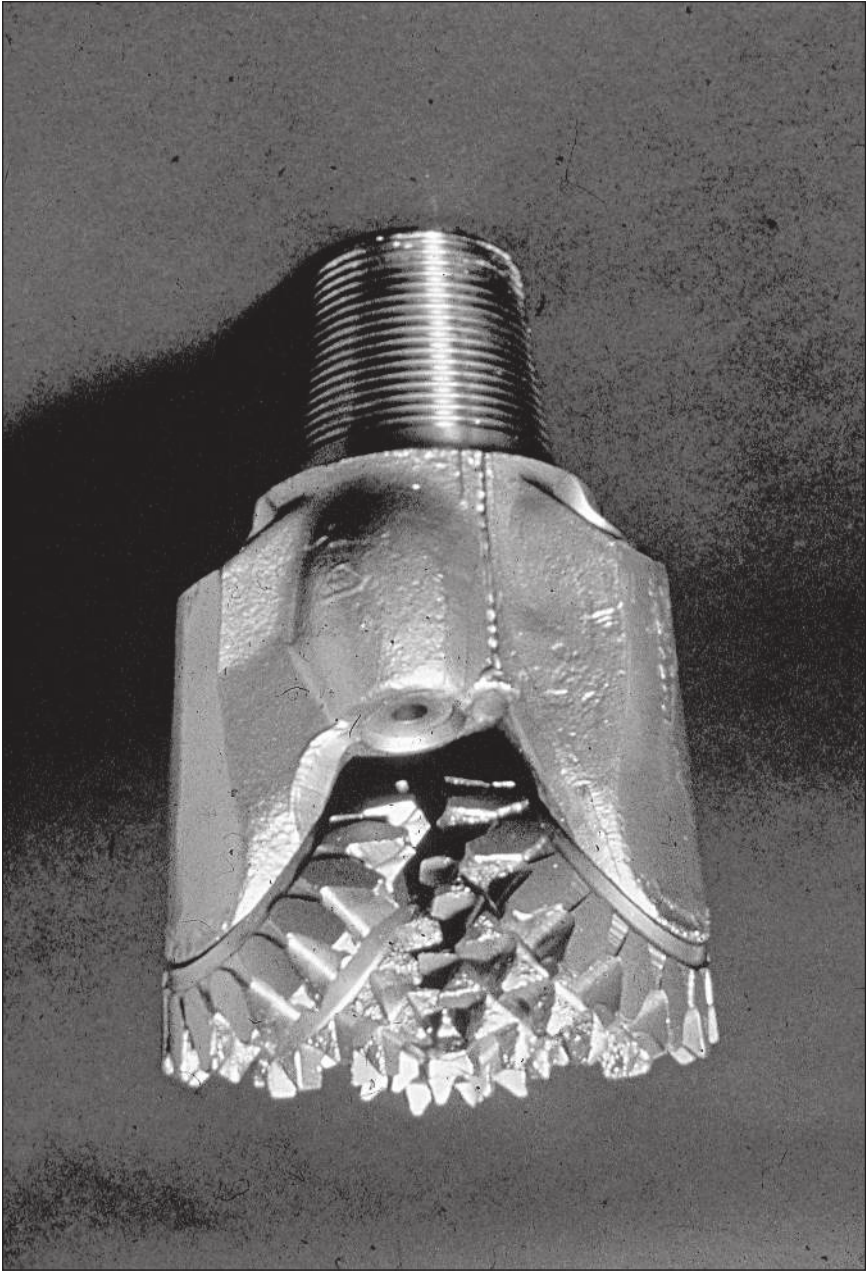
Plate 15–4. Milled-teeth tricone drill bit. (Courtesy of API.)
