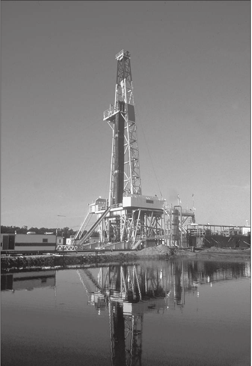
Plate 14-2. Wildcat well being drilled by a modern rotary drilling rig. (Courtesy of Parker Drilling.)
