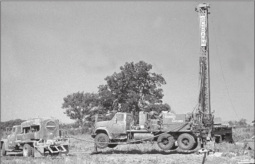
Plate 17-1. Truck-mounted air drilling rig. Note the smaller truck with an air compressor to the left. The blooie line is pointing out from the bottom of the drilling rig.
