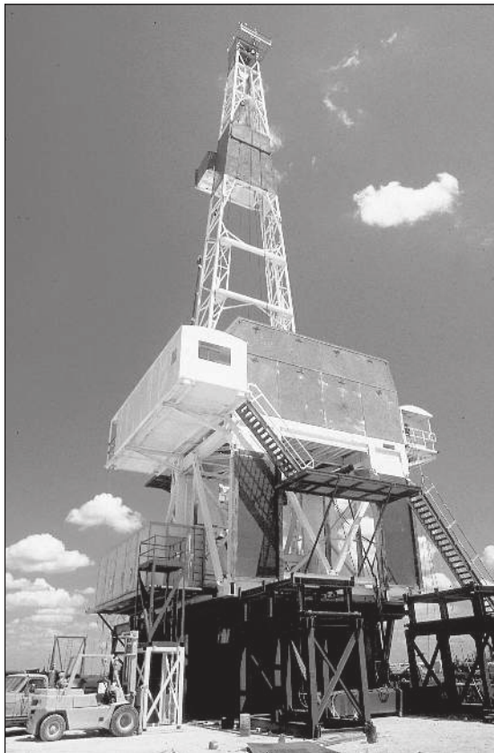
Plate 15-1. Rotary drilling rig. (Courtesy of Parker Drilling.)
