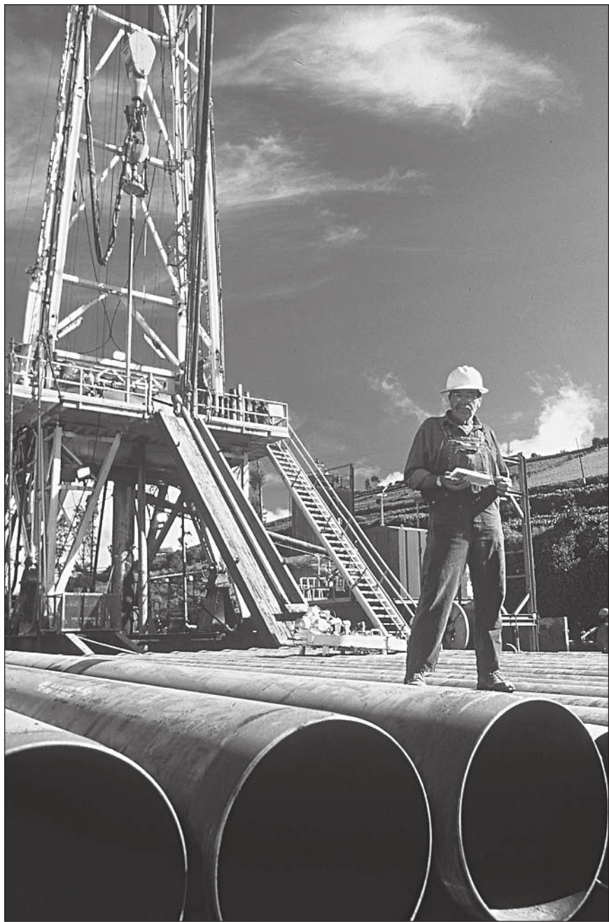
Plate 19–1. Casing racked in front of a well. (Courtesy of Parker Drilling.)
