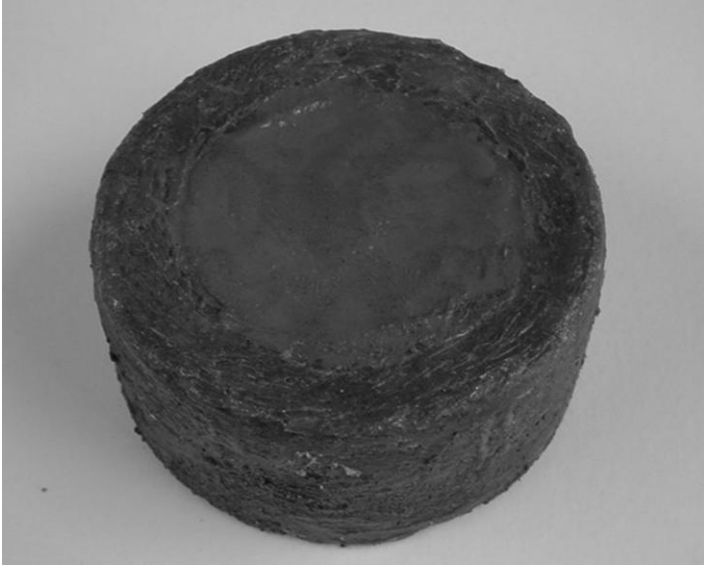
15.14 The set-up of bottom layer mix and compacted clay with silicone rubber round the rim and inside wall to prevent ingress of leachate from rim and interfaces.
