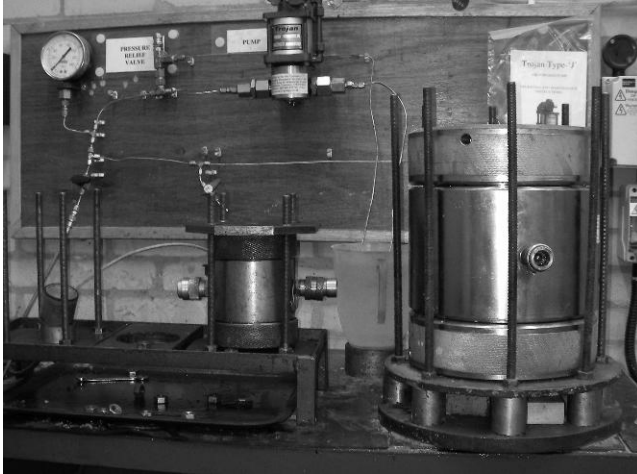
4.4 High pressure apparatus at Coventry, showing one small cell (for 54 mm diameter samples) and one big cell (for 100 mm diameter samples) together with the frame for the second small cell, the liquid pump and pressure gauge.
