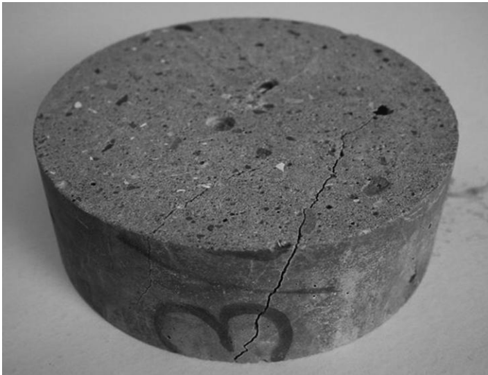
15.12 Narrow cracks induced in the fibre-reinforced mortar disc.
