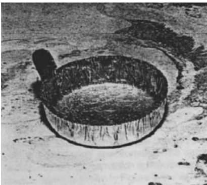
FIGURE 22.2 Crackle test for water using a small aluminum foil cup on a hot plate. Sputtering indicates water contamination.
