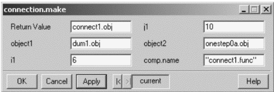
FIGURE 3.29 Filled-in GUI for connecting states 6 with 10 of a previously constructed creep process ( Figures 3.5 and 3.6 ) using a single arrow.
