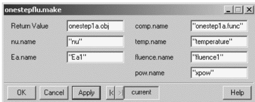
FIGURE 3.11 Filled-in GUI for one-step process, combined Arrhenius, and power-law dependence.
