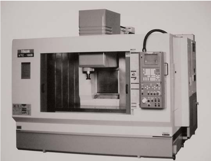
Figure 8 Three Axis Machining Center Courtesy MAZAK Corporation
