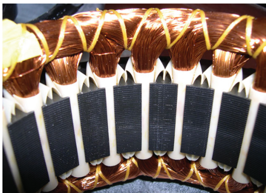
Fig. 5.1. Stator of an AC machine with winding distributed in slots.
