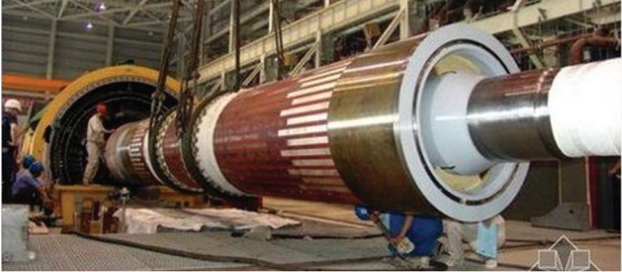
Fig. 7.4. Non-salient pole rotor of a large turboalternator. The end turns are protected against centrifugal and electrodynamic forces with the aid of sleeves made of nonferromagnetic material.
