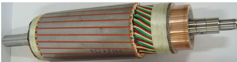
Fig. 4.5. Rotor of a DC brush machine with armature winding inserted in slots, commutator and shaft.
