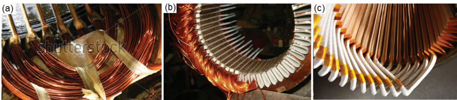
Fig. 5.11. Different techniques of stator coil winding: (a) concentric coils wound of round wire; (b) lap winding wound of round wire; (c) lap winding made of stiff diamond-type coils.
