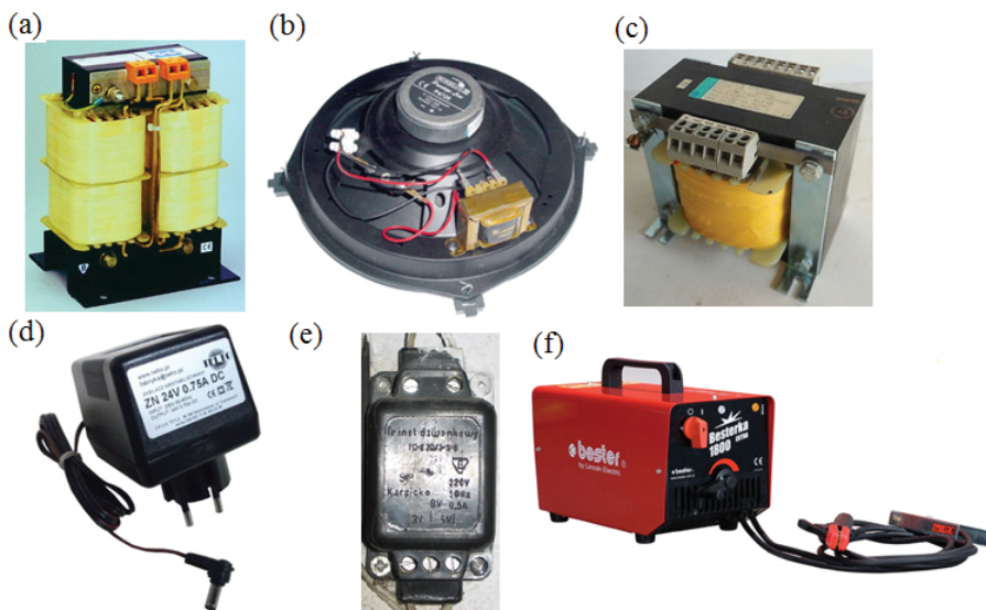
Fig. 2.5. Single-phase air cooled transformers: (a) separation transformer; (b) loud-speaker transformer; (c) radio transformer; (d) step-down transformer with rectifier; (e) door bell transformer; (f) welding transformer.
