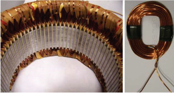
Fig. 5.9. Winding made of elastic coils inserted in slots or sewed up: (a) stator; (b) coil.
