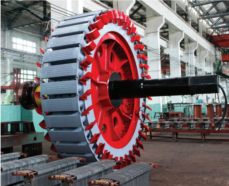
Fig. 7.5. Salient-pole rotor of a hydrogenerator. Below the rotor on the floor, there are salient poles with cage damper winding.
