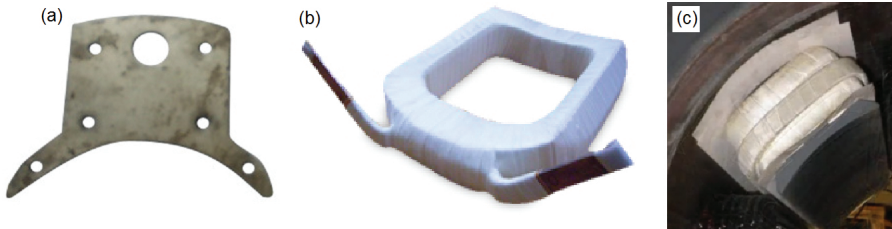
Fig. 4.11. Construction of main poles and field excitation coil: (a) punching (pole core with pole shoe); (b) field excitation coil; (c) main pole with field coil.
