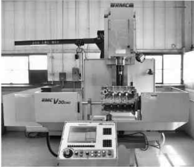
Figure 10.12 Honing surface for cylinder using RMC V30 4-axis CNC [34].
