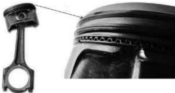
Figure 10.8 Coated piston ring using Diamond [30].
