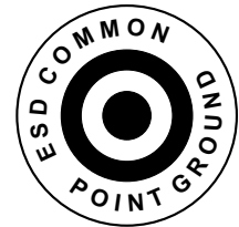
Fig. 13.43 Symbol for ESD common point ground
