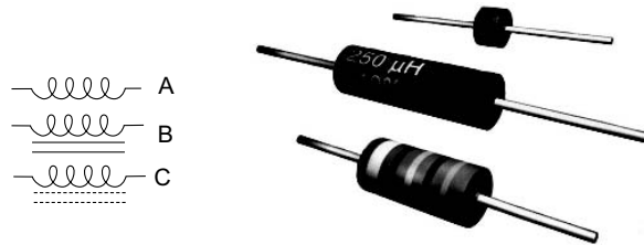
Fig. 2.26 (a) symbol of inductor (b) packages of inductors
