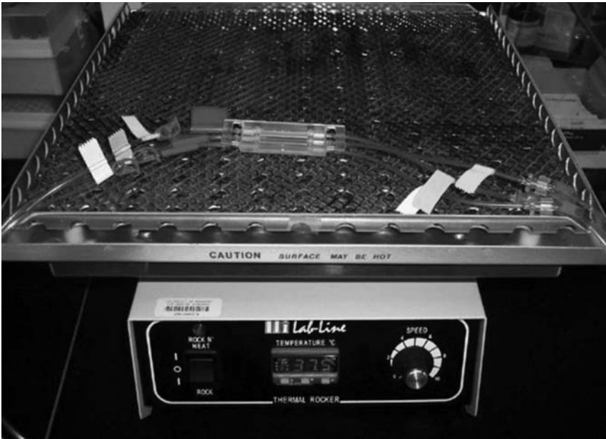
Fig. 10. After inoculation, the flow cell chamber is placed upside down in a 37°C incubator. Growth at 37°C is maintained without medium flow for 1 h, after which the flow cell is returned to an upright position and medium flow is resumed.
