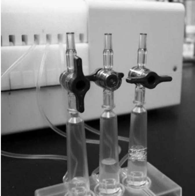
Fig. 7. Bubble traps in the flow cell apparatus are sequentially filled by turning a bubble trap stopcock to the “on” position. Each bubble trap cylinder is filled approximately half full with medium, and then the bubble trap stopcock is returned to the “off” position. This process is repeated for each of three bubble traps per flow cell.
