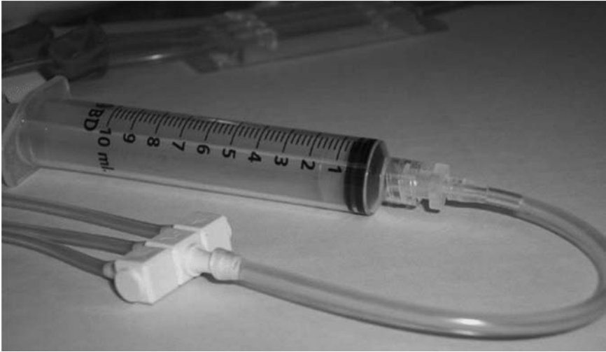
Fig. 2. A 20-mL sterile “male” Luer-Lok fitted syringe is connected to a small (~6 in.) section of sterile tubing by means of a “female” Luer-Lok adapter. The other end of the sterile tubing is subsequently attached to the flow cell output manifold. This apparatus is used to introduce plasma into the flow cell circuit.
