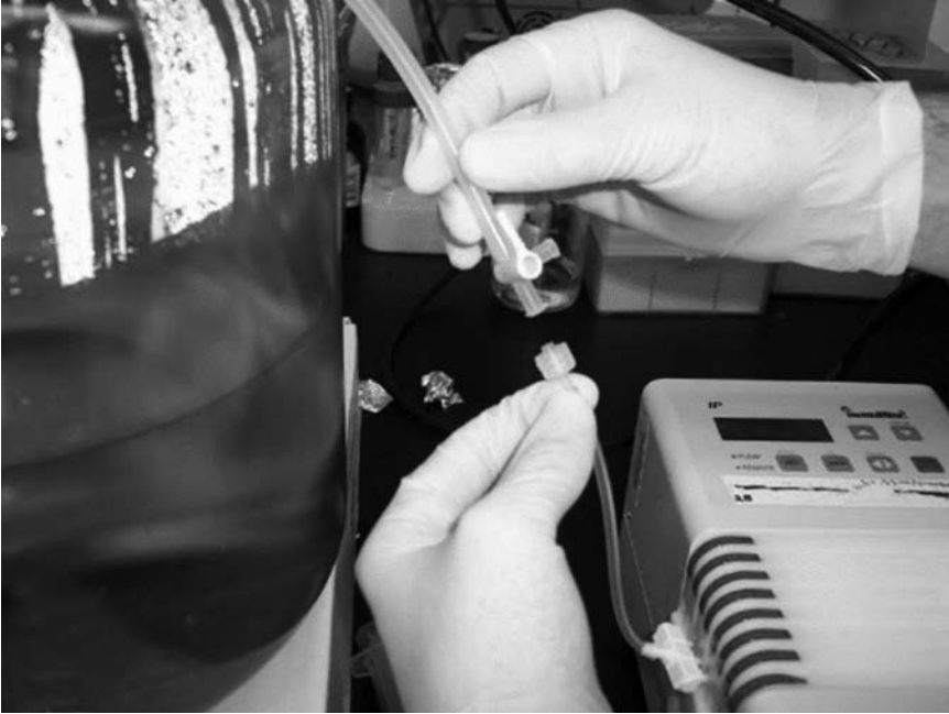
Fig. 5. The “female” Luer-Lok adapter on the section of tubing connected to the flow cell input manifold is removed and replaced with a “male” Luer-Lok adapter. The flow cell may now be aseptically connected to the sterilized media reservoir by means of the three-way stopcock.
