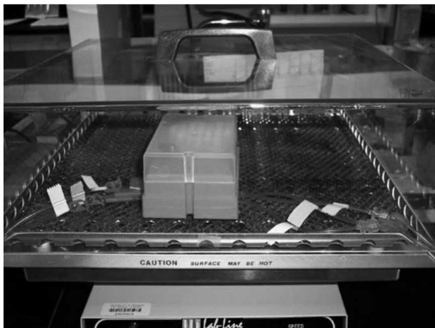
Fig. 11. The flow cell tubing should not be impacted as it enters or exits the incubator. The flow cell chamber should be level with the incubator surface at all times throughout the experiment (a small weight may be used for this purpose).
