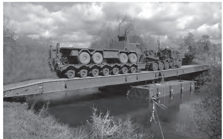
Figure 12.12 Loaded heavy equipment transporter crossing a 46m two-span aluminium alloy military bridge supported at midspan by a floating aluminium alloy pontoon pier
