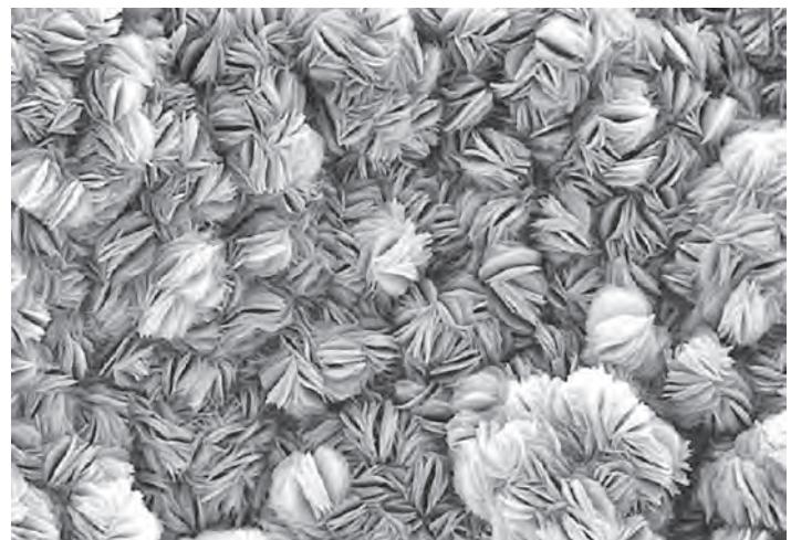
Figure 24.8 Expansive ASR crystals (EM) (photograph courtesy of LCPC)
