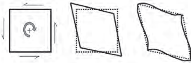
Figure 11.7 Distortion and warping of a box girder
