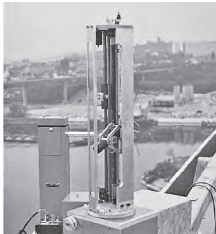
Figure 24.44 Laser deflectometer: a stationary laser beam emission source (left) fixes the position of the target, a beam receiver cell mounted on a trolley (right), which, being brought to a standstill, has a sliding vertical track linked to a point on the bridge; after an initial reading, the relative sliding vertical distance is the deflection of that point on the bridge (photographs courtesy of LRPC Nancy)
