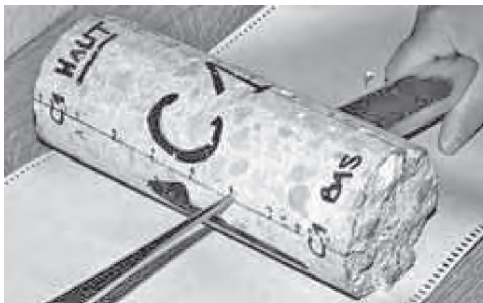
Figure 24.23 Sonic test on concrete sample (photograph courtesy of LRPC Lyon)
