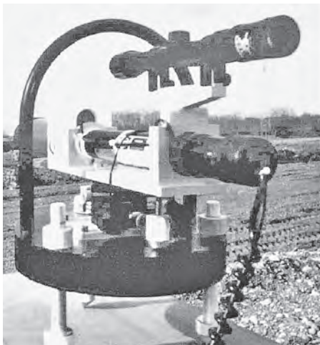
Figure 24.44 Laser deflectometer: a stationary laser beam emission source (left) fixes the position of the target, a beam receiver cell mounted on a trolley (right), which, being brought to a standstill, has a sliding vertical track linked to a point on the bridge; after an initial reading, the relative sliding vertical distance is the deflection of that point on the bridge (photographs courtesy of LRPC Nancy)
