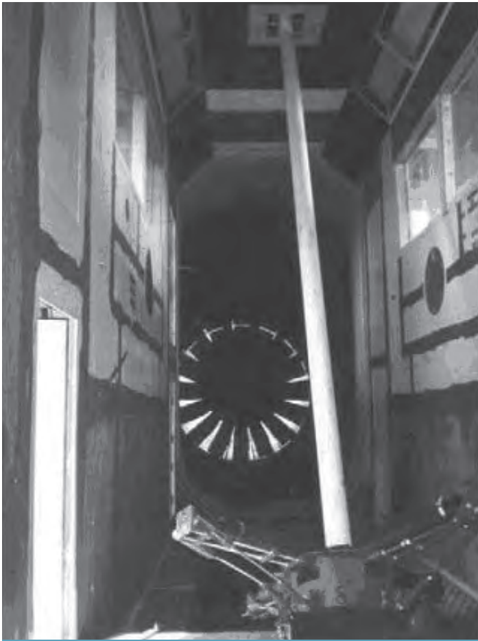
Figure 5.19 Wind tunnel testing of stay cable
