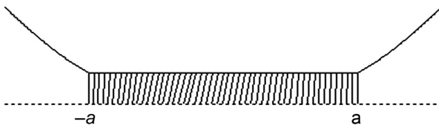
FIGURE 2.42 Brush deflections along the contact area for pure brake slip.
