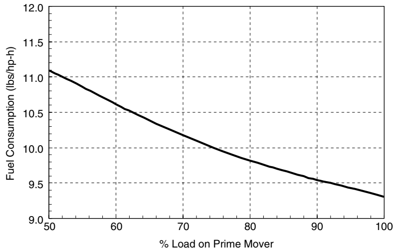
Figure 11.8 Fuel consumption of prime movers using natural gas as fuel.
