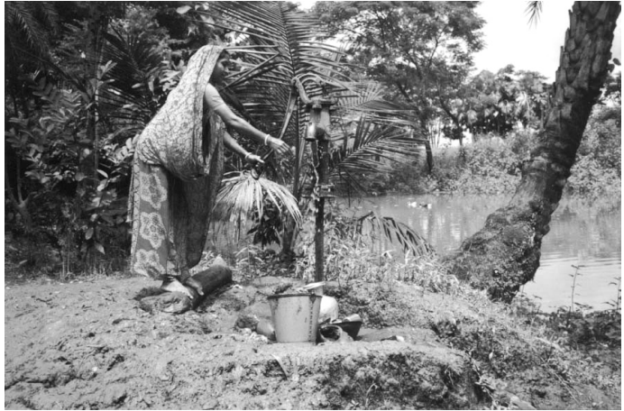
FIGURE 9.9 Manually operated water pump
