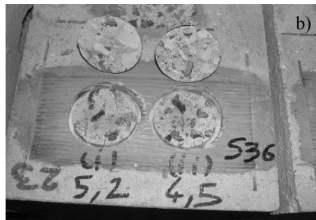
Figure 24.13. Results of the pull-off tests for CFS strengthened blocks: pull-off strength versus ageing time (a) type of substrate failure observed both in the initial and aged states (b)
