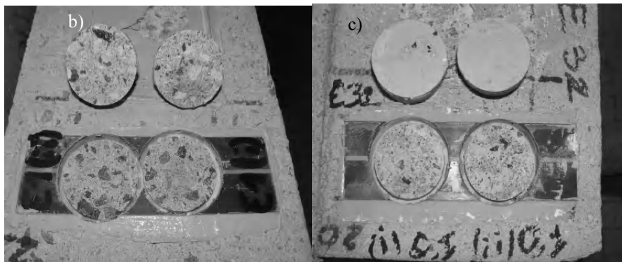
Figure 24.10. Results of the pull-off tests for CFRP strengthened blocks: pull-off strength versus ageing time (a) and pictures of fractured surfaces in the initial (b) and aged (c) states
