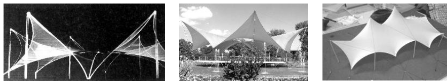
Figure 14.7. Physical model: soap film and achieved membrane (Tanzbrunnen, Cologne); fabric model
