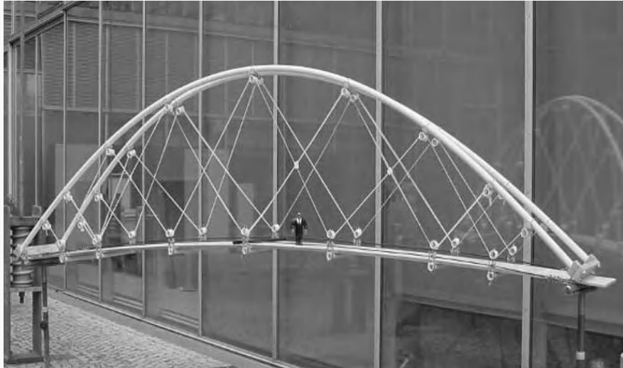
Figure 13.3. Composite bowstring, scale 1/10 (ENPC)
