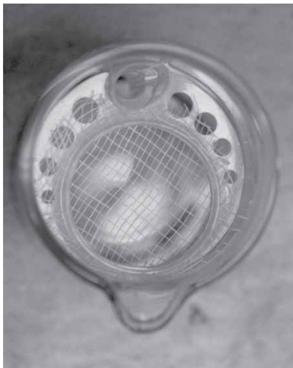
Fig. 2. Top view of slice-holding chamber. Note the Lexan insert with holes for the chimney and the slice platform. A drilled-out plastic Petri dish mates with the insert to lock down a single layer of cotton 4 \times 4 to provide a broad net to hold the slices without impeding solution flow through the slices. The extra holes in the insert are decorative.
