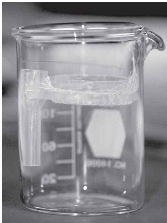
Fig. 1. Side view of slice-holding chamber. Chamber consists of a platform for holding slices and a chimney made from a plastic disposable pipet. Solution completely covers the platform and the top of the chimney. A bubbler in the chimney oxygenates the solution. Bubbles in the chimney produce a gentle flow of solution past the slices.
