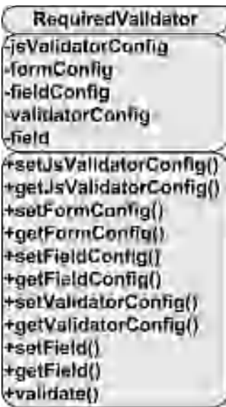
Figure 8-16. UML diagram of the RequiredValidator class
