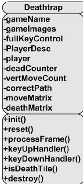
Figure 11-16. UML diagram of the Deathtrap class
