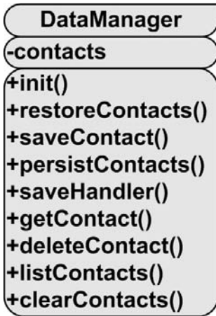
Figure 6-13. UML diagram of the DataManager class
