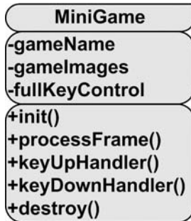
Figure 11-10. UML diagram of the MiniGame class
