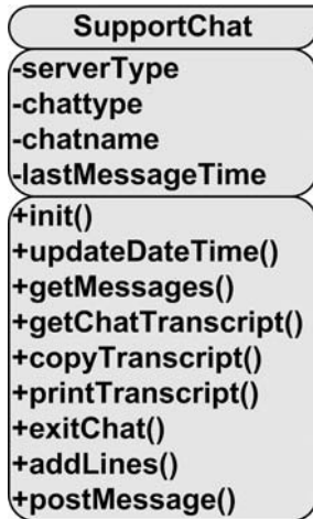
Figure 12-6. UML diagram for the SupportChat class
