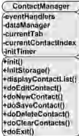
Figure 6-12. UML diagram of the ContactManager class
