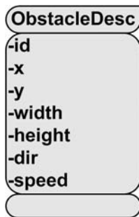
Figure 11-13. UML diagram of the ObstacleDesc class
