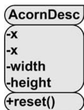
Figure 11-15. UML diagram of the AcornDesc class
