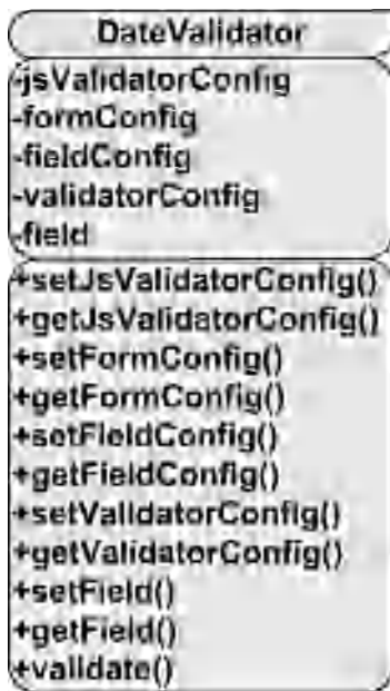
Figure 8-19. UML diagram of the DateValidator class
