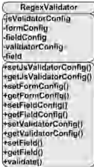
Figure 8-17. UML diagram of the RegexValidator class
