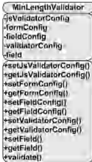
Figure 8-18. UML diagram of the MinLengthValidator class
