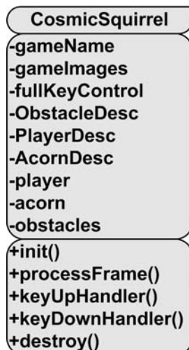
Figure 11-12. UML diagram of the CosmicSquirrel class
