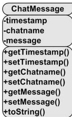
Figure 12-9. UML diagram of the ChatMessage class
