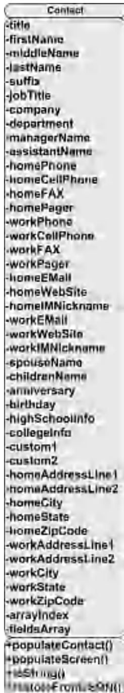
Figure 6-11. UML diagram of the Contact class
