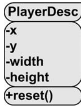
Figure 11-14. UML diagram of the PlayerDesc class
