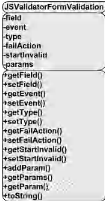
Figure 8-12. UML diagram of the JSValidatorFormValidation class
