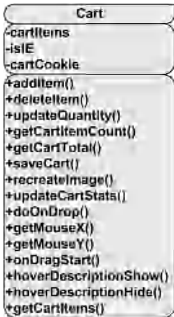
Figure 10-11. UML diagram of the Cart class
