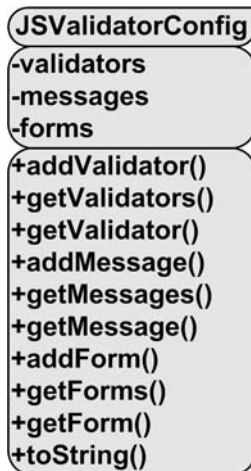
Figure 8-8. UML diagram of the JSValidatorConfig class
