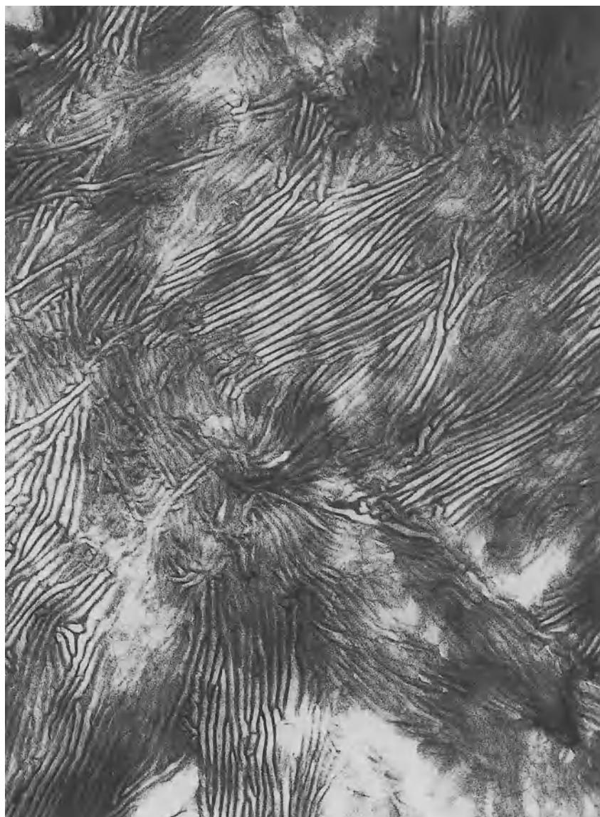
Fig. 8.3. Electron micrograph of an ultrathin section of a polyethylene sample (LPE). The weight average (3.12) of the sample was \langle m \rangle_w = 100\,000 . The sample was annealed at 125 °C for four weeks, subsequently stained with chlorosulphonic acid at 60 °C for five hours, and finally treated with uranyl acetate at room temperature [Kanig (1991), Fig. 1]. The enlargement was 1:50 000
