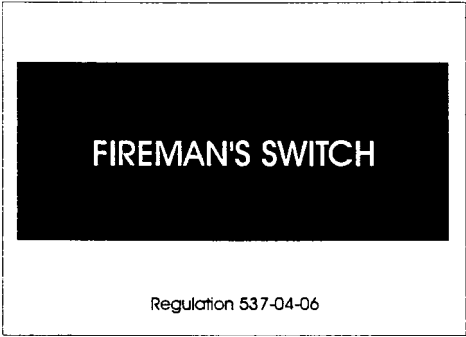
Figure 9.19: Fireman's switch notice
