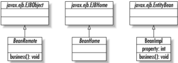
Figure 1-11. The EJB component model
