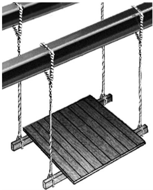
FIGURE 31.3 Interior-hung scaffold. (Source: Occupational Safety & Health Administration, Washington, DC.)
