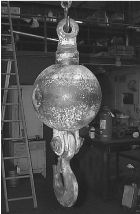
FIGURE 16.17 Typical swivel and headache ball, attached to hook. (Source: Gunnebo Johnson Corp., Tulsa, OK.)
