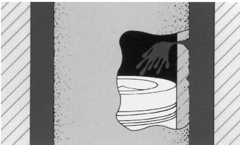
12-9 Cavitation erosion results in coolant leaks into the cylinders.
