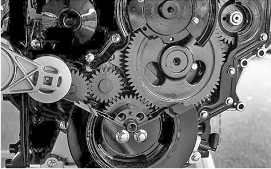
2-9 The Cummings ISB employs straight-cut timing gears that, while noisy, are practically indestructible. Gilmer-type toothed timing belts, typical of passenger-car diesels, need replacement at 60,000 miles or less.
