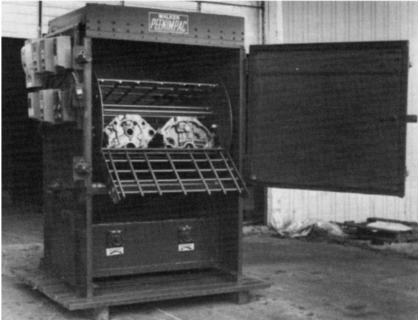
7-20 Walker Peenmatic shot blaster adds an “as-new” finish used casting.
