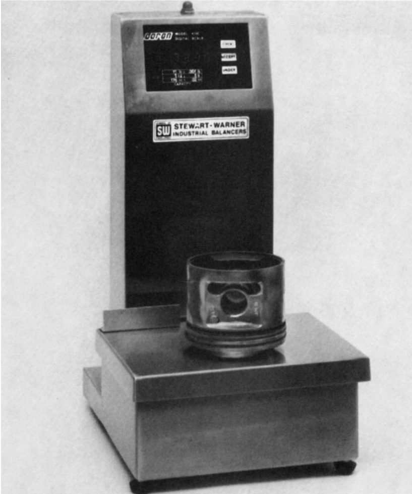
8-79 Balancing begins with match-weighing piston assemblies.
