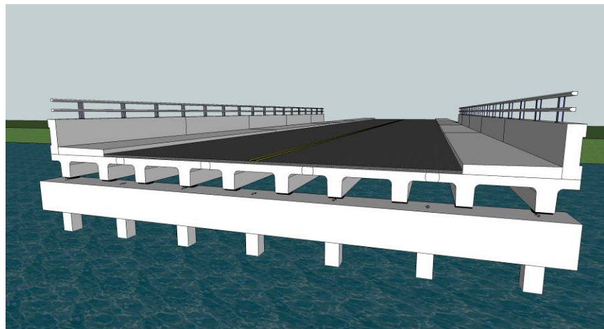
Figure 5.2.4.2-1 Adjacent Deck Double Tee Beam Superstructure
