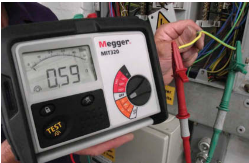
Figure 4.35 Test each end of the CPC
