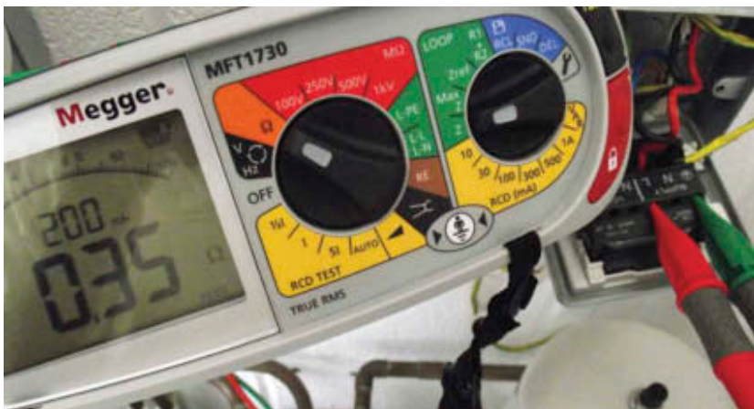
Figure 4.55 Test between line and earth R_1 + R_2
