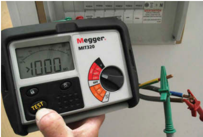
Figure 4.47 Join live conductors and test to earth
